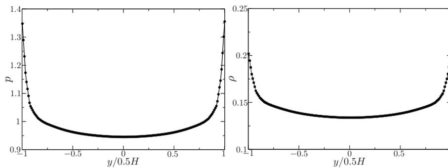
Figure 2: One-dimensional vertical plots of the flow field at  $x = 0$ . a) Pressure [bar] as a function of normalized coordinate. b) Density [kg/m<sup>3</sup>] as a function of normalized coordinate.  $E_a = 0$ ,  $L = L_{ref}$  et  $H = H_{ref}$ .
