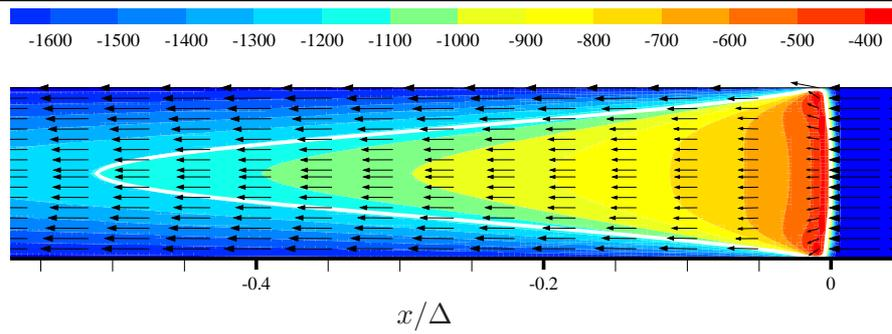
Figure 1: Longitudinal velocity [m/s] flow field in the shock-attached frame. The white line indicates the sonic condition.  $E_a = 0$ ,  $L = L_{ref}$ ,  $H = H_{ref}$ .
