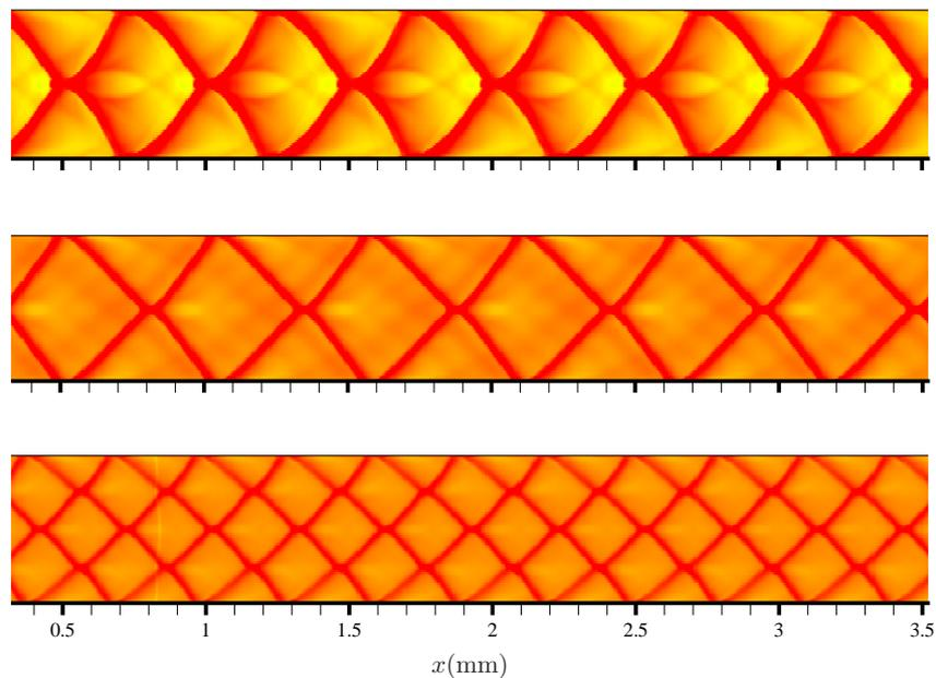
Figure 3: Maximum pressure histories for various activation energies. From the bottom to the top:  $E_a = 0$ ,  $E_a/\mathcal{R}T_0 = 10$  and  $E_a/\mathcal{R}T_0 = 20$ .  $L = L_{ref}$ ,  $H = 4H_{ref}$ .
