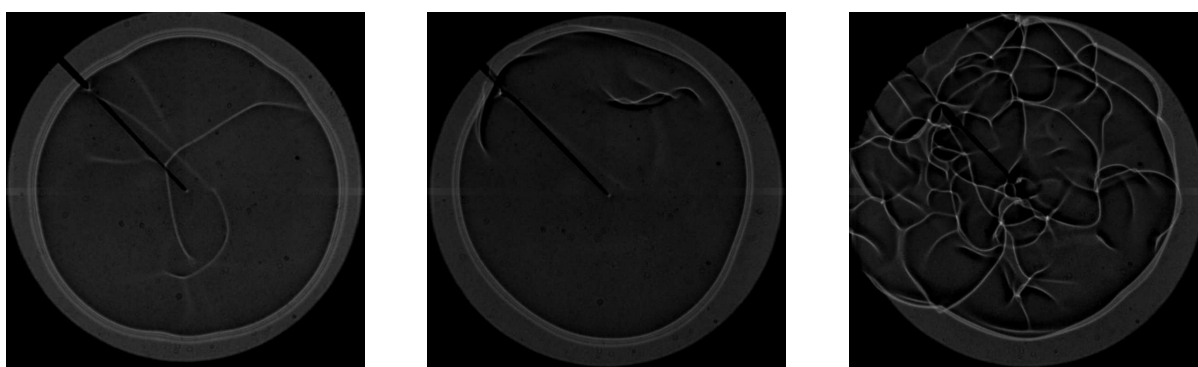
Figure 3: Examples of shadowgraph frames. Left: methane-air-water flame aerosol at near-stoichiometry. Middle: propane-air-water flame aerosol at \phi = 0.7 . Right: propane-air-water flame aerosol at \phi = 1.3 .
