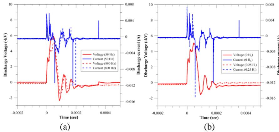
Figure 2. Typical voltage and current curve of pulsed-DC SECD showing several microdischarges. The pulse duration is 100 μs. Red lines represent discharge voltage, and blue lines represent discharge current. (a) for various PRFs at electrode located height of 0 H<sub>L</sub>. (b) for various electrode located heights with PRF of 800 Hz.
