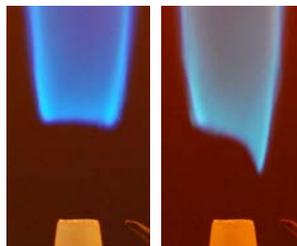
Figure 3. Photographs of lifted flames without (left) and with (right) pulsed discharges for jet exit velocity of 7.9 m/s and PRF of 800 Hz. The located height of electrode is 0 H<sub>L</sub>. The lifted flame base with a cusp-like shape in the discharge case.
