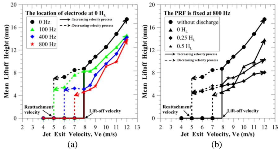
Figure 4. Mean liftoff height versus jet exit velocity for (a) various PRFs of 0, 100, 400 and 800 Hz at the electrode-located height of  $0 H_L$ . (b) various electrode-located heights of 0, 0.25 and 0.5  $H_L$  with a PRF of 800 Hz.
