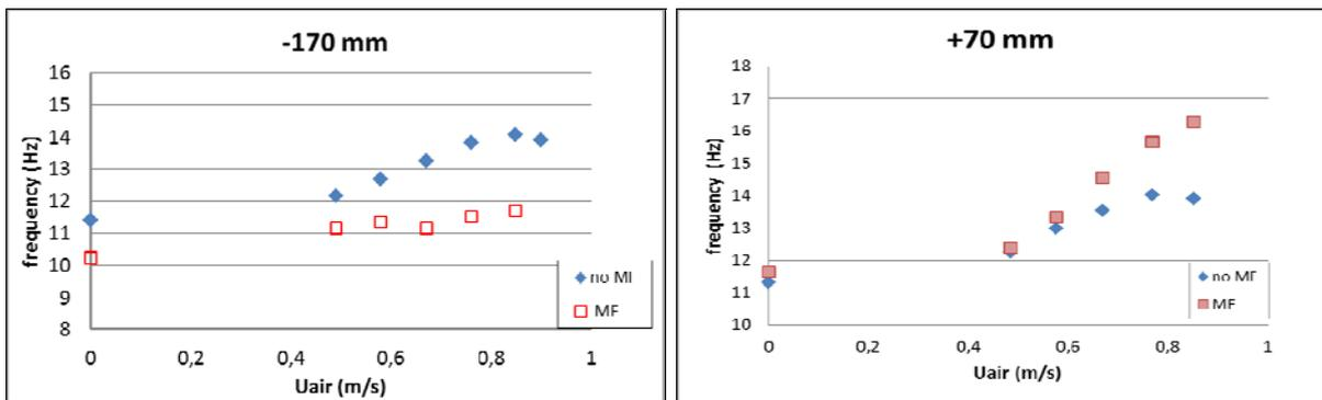
Figure 4. Flickering frequency versus air injection velocity without (no MF) and with magnetic gradient (MF) in the two burner positions.
