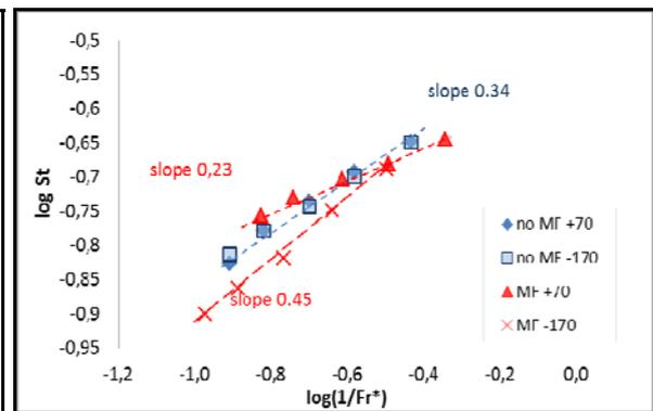
Figure 6. Relation between the Strouhal number and the inverse Froude number without and with positive (-170mm) and negative (+70 mm) magnetic gradients.
