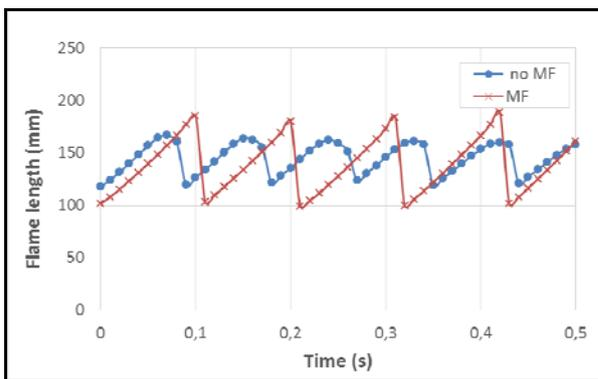
Figure 5. Time variation of the flame length along 0.5 s for the case of  $U_{air}=0$  and position of the burner in the magnetic bore  $z = -170$  mm.
