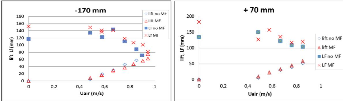
Figure 3. Flame lift height and flame length versus air injection velocity without (no MF) and with magnetic gradient (MF) in the two burner positions.
