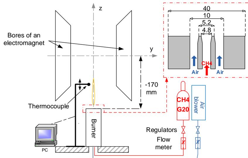
Figure 1. Experimental setup and burner geometry
