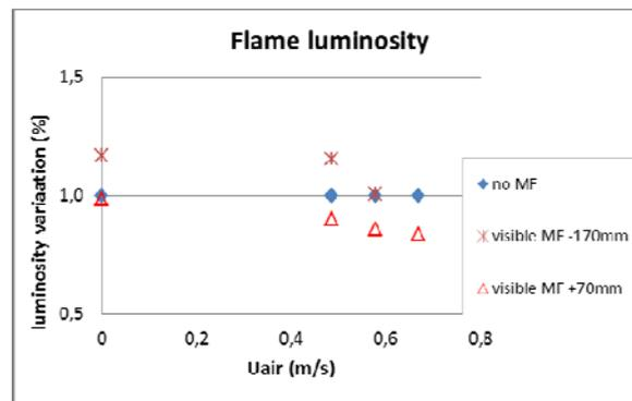
Figure 7. Comparison of natural flame luminosity variation without (no MF) and with magnetic gradient (MF) in the two burner positions at different air injection velocity
