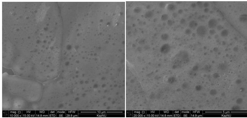
Figure 2 – Samples of the surface of the granules of ammonium nitrate on scanning electron microscope (SEM)
