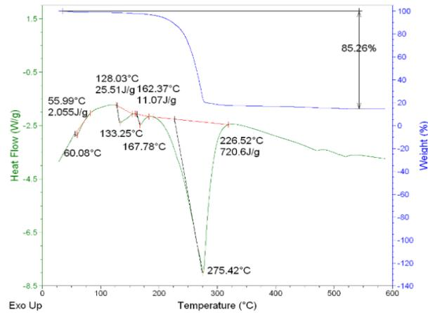
**Figure 6** – DSC curves and thermal decomposition of  $\text{NH}_4\text{NO}_3$ /Dextran 20 wt. %.
