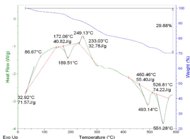
**Figure 4** – DSC curves and thermal decomposition of dextran under argon environment.
