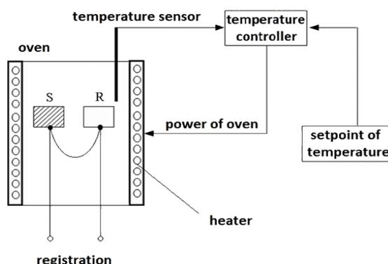
**Figure 1** – Experimental setup of the Differential Scanning Calorimetry (DSC) and Thermogravimetric Analyzer (TGA)
