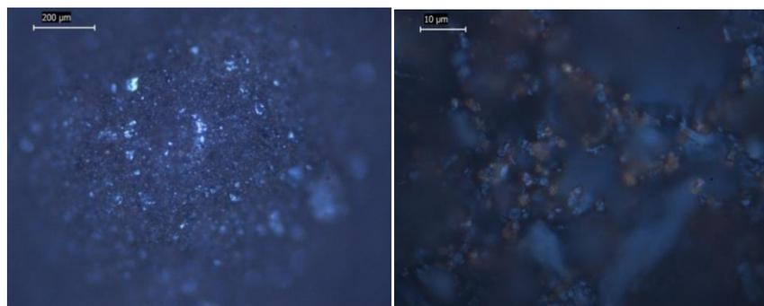
Figure 3 – Samples of surface of the mixture ammonium nitrate and the dextran by optical microscope.
