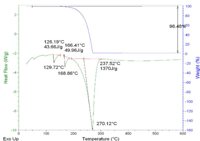
**Figure 5** – DSC curves and thermal decomposition of  $\text{NH}_4\text{NO}_3$  under argon environment.
