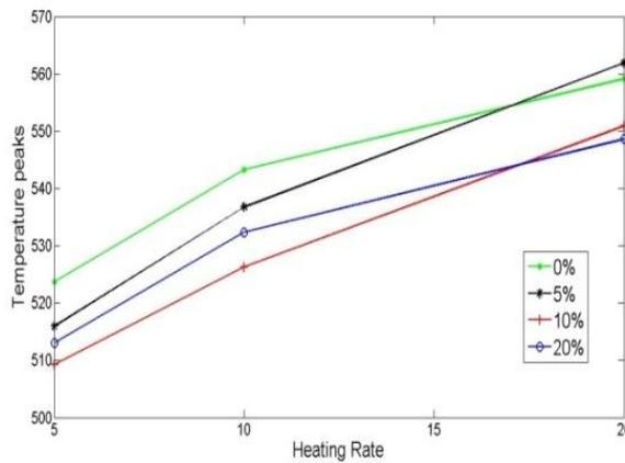
**Figure 8** – Dependence of decomposition temperature of  $\text{NH}_4\text{NO}_3$  and  $\text{NH}_4\text{NO}_3$ -dextran on a heating rate
