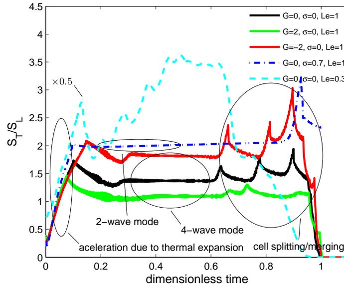
Figure 4: The reduced front speed with the dimensionless time for 5 cases. Solid curves: (centre) for  $G = 0, \sigma = 0, Le = 1$ ; (down) for  $G = 2, \sigma = 0, Le = 1$ ; (up) for  $G = -2, \sigma = 0, Le = 1$ . Dashed curve: for  $G = 0, \sigma = 0, Le = 0.3$ . Dot-dashed curve: for  $G = 0, \sigma = 0.7, Le = 1$ .
