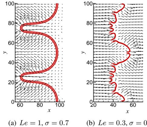
Figure 3: Flame fronts represented by the reaction rate contours and the flow velocity vectors calculated for a)  $Le = 1, \beta = 10, \gamma = 5, \sigma = 0.7, G = 0$  and b)  $Le = 0.3, \beta = 10, \gamma = 2.5, \sigma = 0, G = 0$ .
