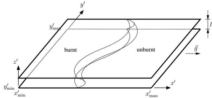
Figure 1: Sketch of the Hele-Shaw cell with a curved flame propagating from the left to the right between two parallel plates with a cell gap  $h$ .
