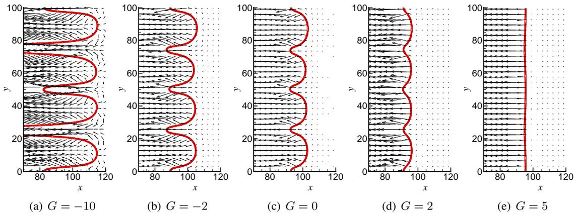
Figure 2: Flame fronts represented by the reaction rate contours and the flow velocity vectors calculated for  $Le = 1, \beta = 10, \gamma = 5, \sigma = 0,$  with increasing values of  $G$  (upward propagation for  $G < 0$  and downward propagation for  $G > 0$ ).
