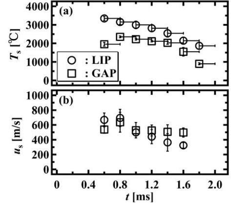
Fig. 4 Measured temperature (a) and speed (b) of CoNiCrAlY powder.
