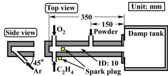
Fig. 1 PDC for the GAP-mode operation.
