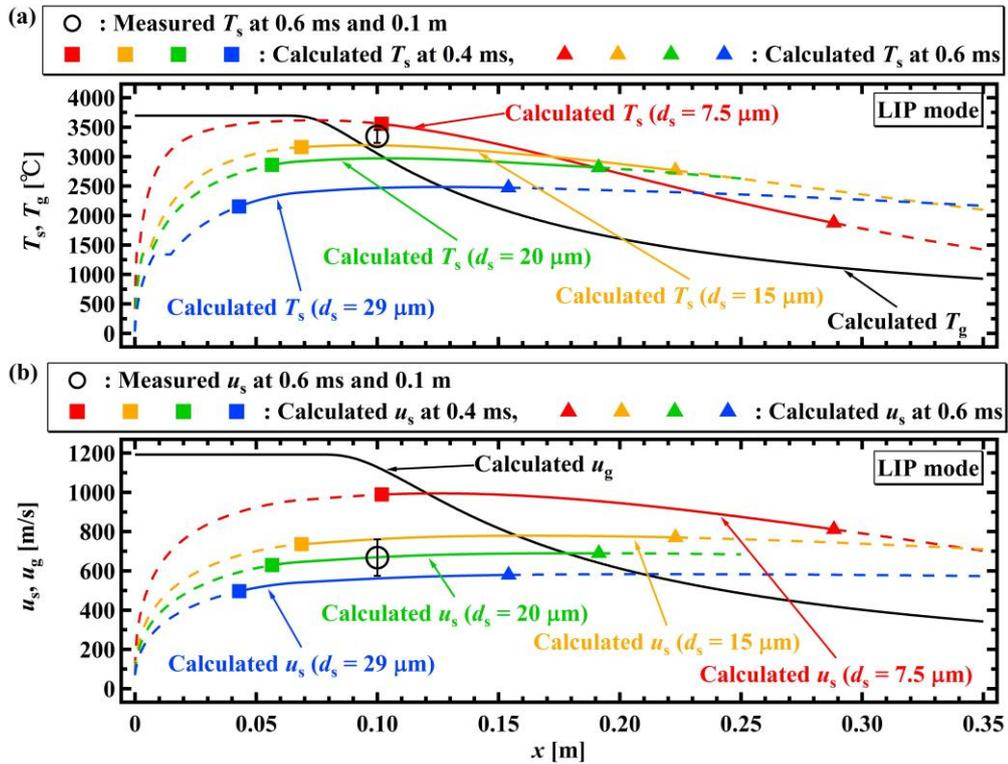
Fig. 6 Comparison of the calculation results with the experimental data for the LIP-mode operation.
