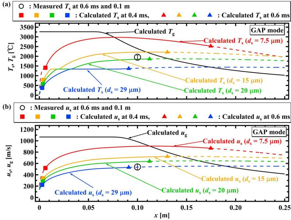
Fig. 5 Comparison of the calculation results with the experimental data for the GAP-mode operation.
