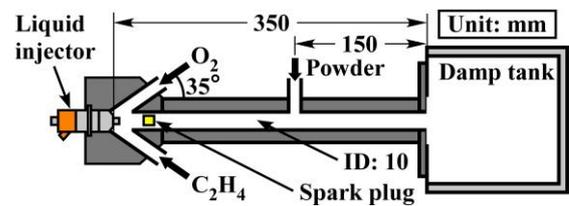
Fig. 2 PDC for the LIP-mode operation.
