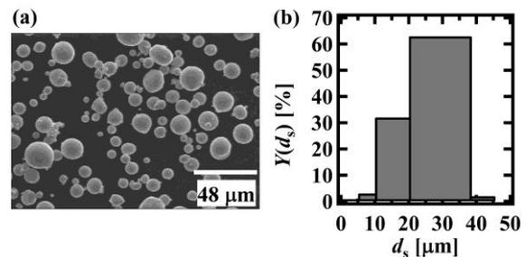
Fig. 3 CoNiCrAlY powder.
