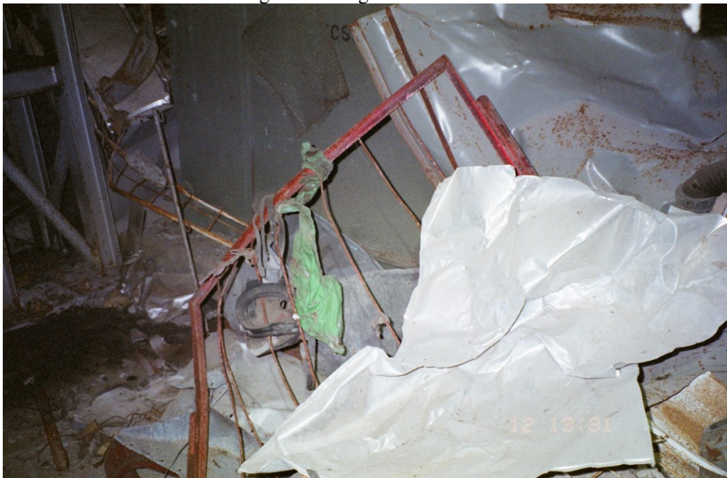
Figure 12 Heat damage on plastic materials
