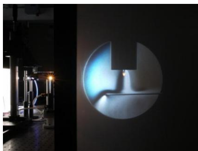
Figure 5 Photograph of the Z-type Schlieren experimental setup on an optical table
