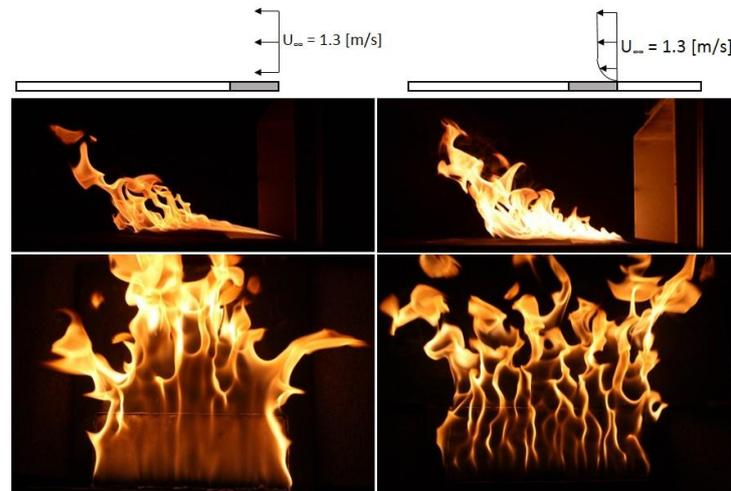
Figure 2: Boundary layer effects on a stationary wind-blown fire. (Left) No boundary layer development surface, i.e. placed directly in the free-stream flow. (Right) 25 cm boundary layer development surface (boundary layer thickness  $\approx 2 \text{ cm}$ ). The fuel source was a heptane-soaked wick and an inert surface was placed downstream for all experiments to observe attachment of the flame.
