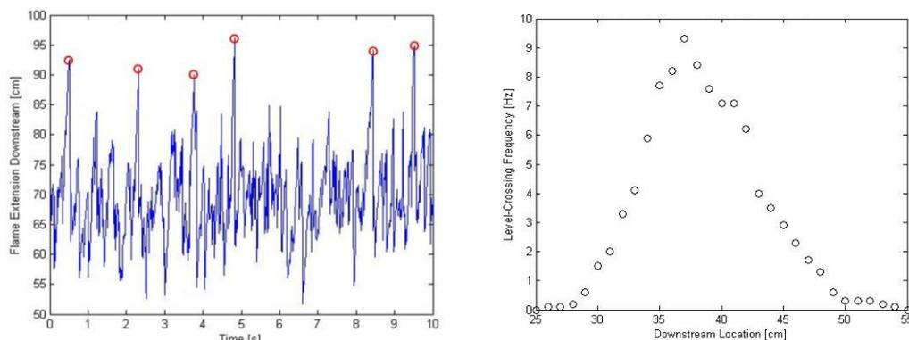
Figure 4: (Left) Flame location over time *from* high-speed videography and (right) VITA frequency at advancing downstream locations. Flame location fluctuates around the maximum frequency pulsation distance, but occasionally “bursts” further downstream (noted by red circles on the left).
