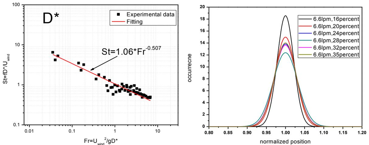
Figure 5: (Left) Strouhal-Froude scaling for stationary burners in a forced-flow environment and (right) occurrence (probability density function) of mean flame position where lpm represents the flow rate of gas and the percentage indicates % free-stream velocity from maximum (~6 m/s).
