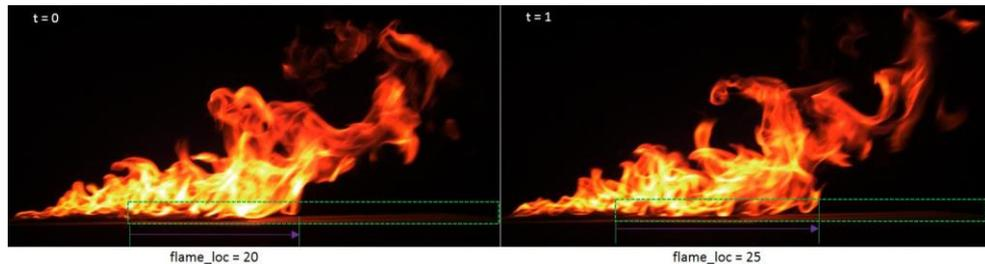
Figure 3: Flame location between two time steps in a forced flow experiment. The flame attachment location ( $x_a$ ) is measured from the downstream edge of the burner to edge of the flame within the attachment region.
