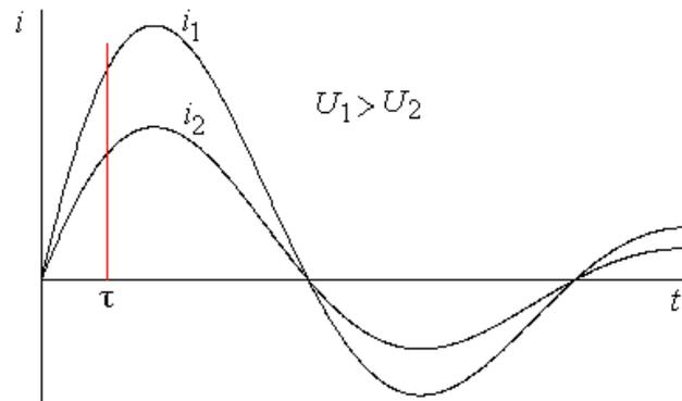
Figure. 8. Correlation between critical time  $\tau$  and discharge currents.
