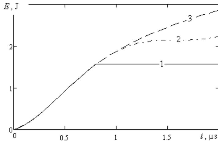
Figure6. The dynamics of energy input into the spark in simulation cases № 1, 2, 3.
