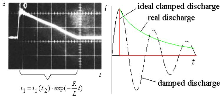
Figure 1. The form of discharge current in case of real [3] (left) and ideal (right) clamping of damped discharge.
