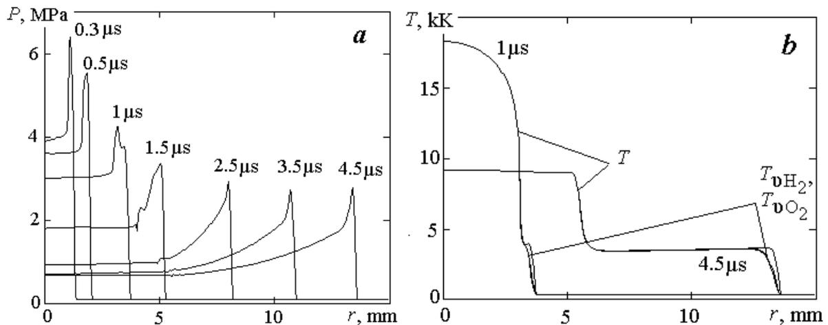
Figure.7. The time histories of pressure (a) and temperature (b):  $T_v$  is vibrational temperature.
