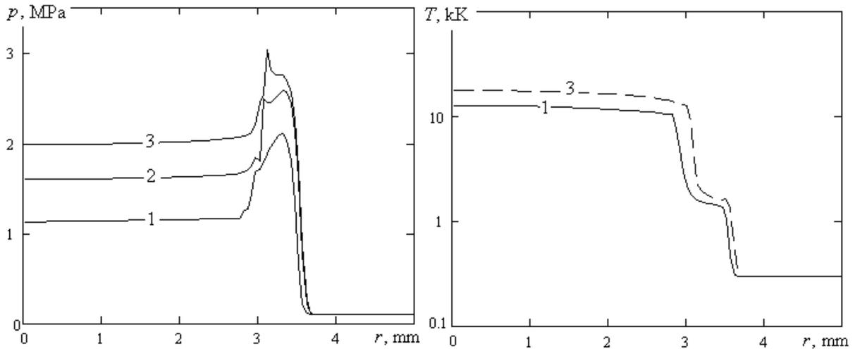
Fig.5. The distribution of pressure (left) and temperature (right) in simulation cases № 1, 2, 3 to the time  $t = 1,6 \mu\text{s}$ .
