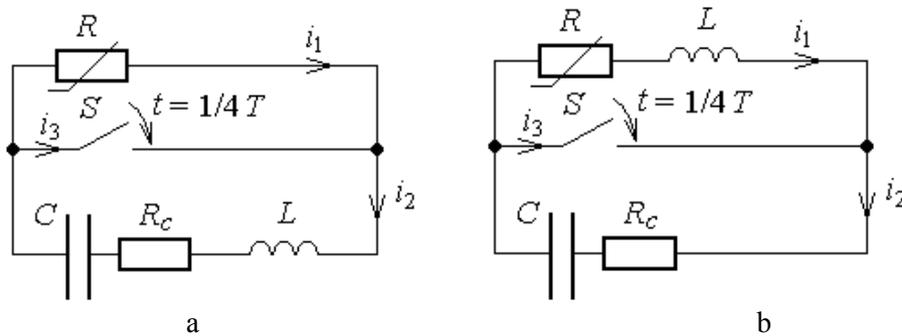
Figure 3. The circuits for ideal (a) and real (b) bridging of the discharge gap in RLC-circuit.
