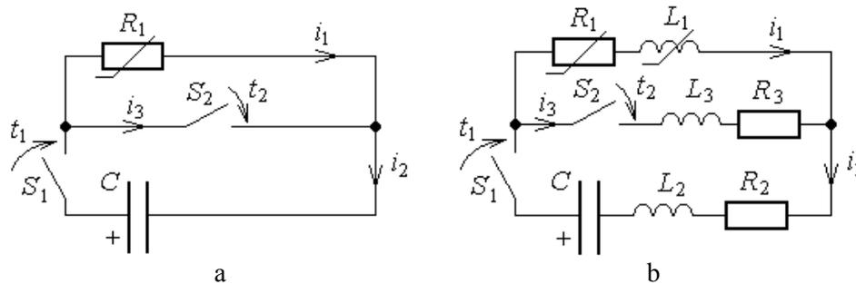
Figure 2. The circuit for bridging the spark discharge (a) and it equivalent electrical circuit (b):  $R$  are active resistances of the spark gap, wires and the internal capacitor resistance;  $C$  is capacitor;  $S$  are electrical switches;  $L$  are inductances of wires, capacitor and discharge gap.
