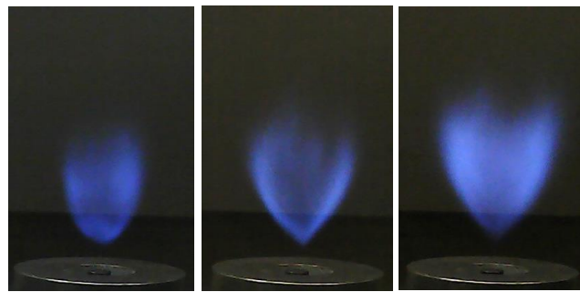
Figure 4. Lift-off height of biogas flame of nozzle N_4
