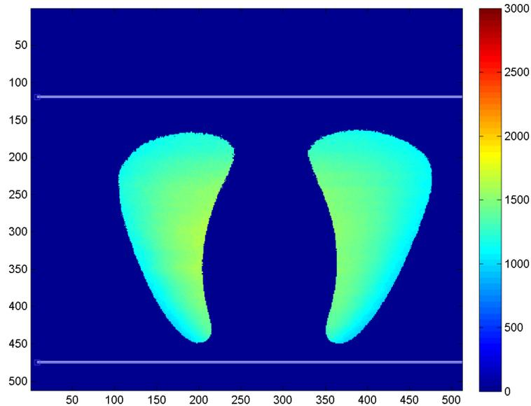
Figure 3 Temperature measurement with a distance plate burner of 9mm; x and y axes show number of pixels
