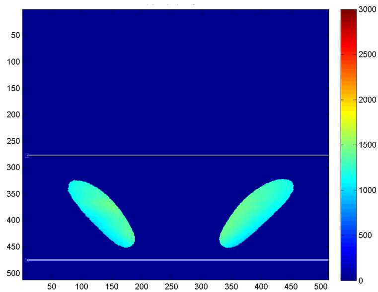
Figure 2 Temperature measurement with a distance plate burner of 5mm; x and y axes show number of pixels
