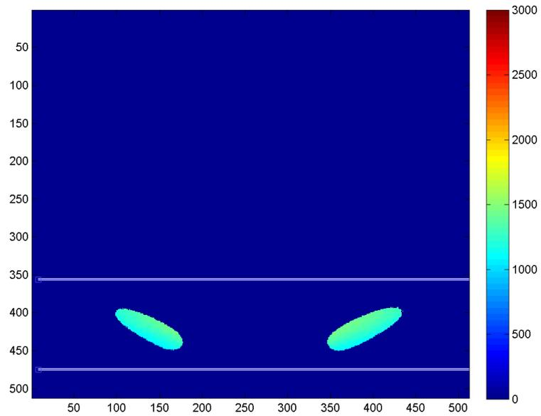
Figure1 Temperature measurement with a distance plate burner of 3mm; x and y axes show number of pixels
