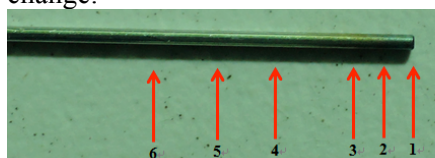
Fig. 7 Photo of the micro stainless steel tube after burning
