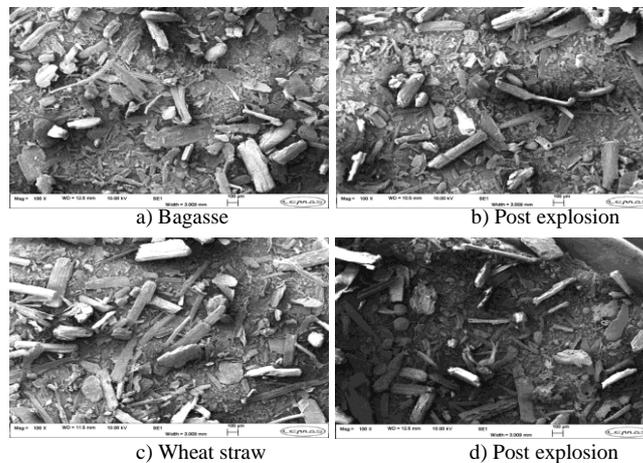
Figure 6. Surface morphology comparison of crop samples and their post explosion residues
