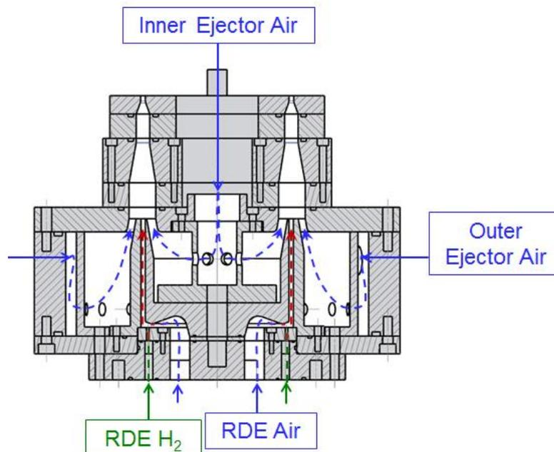
**Figure 1. RDE with ejector cross-section.**
