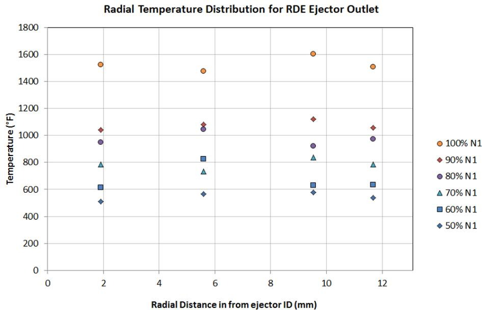
**Figure 4. Radial temperature distribution at ejector outlet plane, for various power settings. Radial location 0 mm represents ejector outlet ID, while Radial location 13.1 mm represents ejector outlet OD.**
