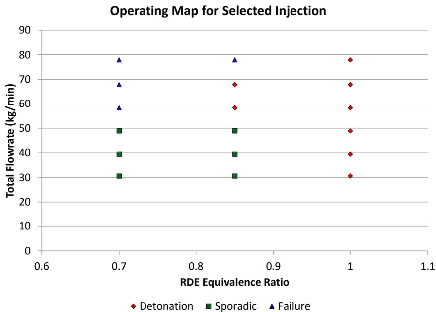
Figure 3. Operating mode as a function of RDE equivalence ratio and total flowrate for selected reactant injection setup.
