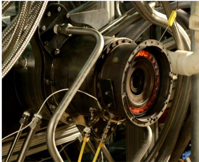
Figure 5. Picture of the T63 RDE assembly running at the 90% power setting.
