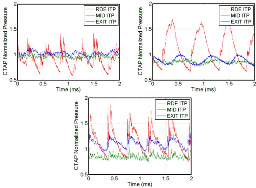
Figure 2. Data samples of sporadic (top left), acoustic (top right), and detonation (bottom) RDE ejector operating modes.
