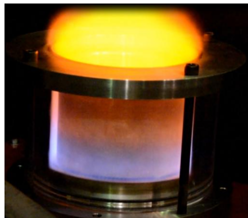
Figure 1. Schematic (left) and photograph (right) of the optically accessible rotating detonation engine.
