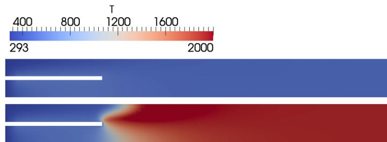
Figure 3. Temperature field in K at  $T_p = 550$  K for the solutions along the ignition branch (top) and extinction branch (bottom).
