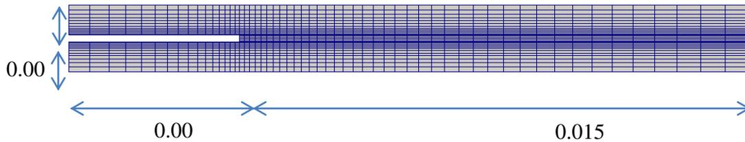
Figure 1. Computational domain and mesh (about 1500 cells). Dimensions are in m.
