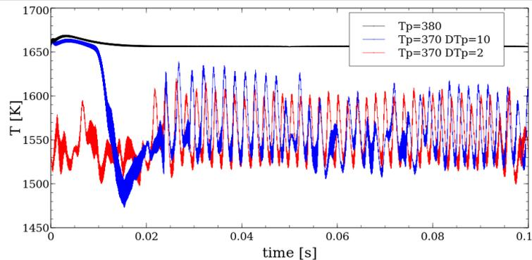
Figure 4. T1 temperatures vs time recorded during the computation of solution on the extinction branch at  $T_p=380$  K, black line, and  $T_p=370$  K, blue line with a single jump of 10 K from  $T_p=380$  K, red line as the result of subsequent computations for  $T_p$  progressively reduced by 2 K jumps from 380 K.
