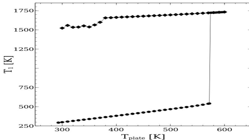
Figure 2. Typical hysteretic behavior representing the ignition and extinction of the system. The  $T_1$  temperature is reported as a function of the temperature of the plate surface.
