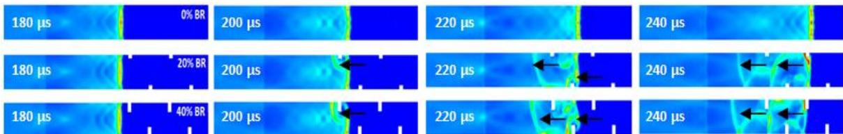
Figure 4. Pressure contours up to 490 mm long part of PDE combustor with all configurations.
