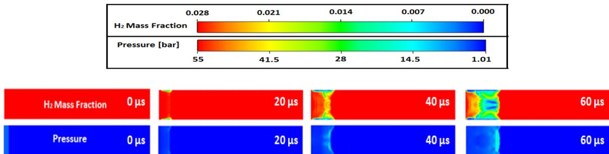
Figure 1. Hydrogen mass fraction and pressure contours plot for 300 mm long part of (0% BR) PDE combustor.
