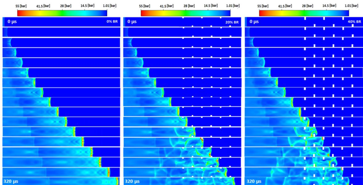
Figure 5. Pressure contours for all configuration of PDE combustor with 600 mm length and 50.8 mm diameter.
