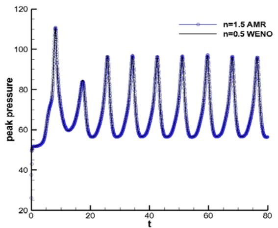
Figure 1. Pressure history at the perturbed ZND shock for one-dimensional plusting detonation.  $n$  is the relative grid size, and there is  $5/n$  grids in half reaction.
