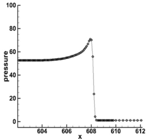
Figure 3. The peak pressure of the ZND shock front in the time domain
