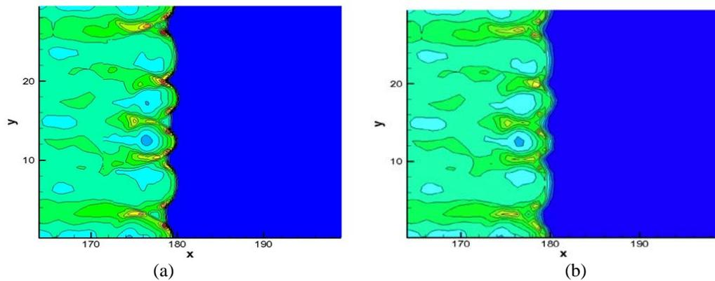
Figure 5. (a) pressure distribution near the detonation front of AMR, the base mesh is  $500 \times 50$
