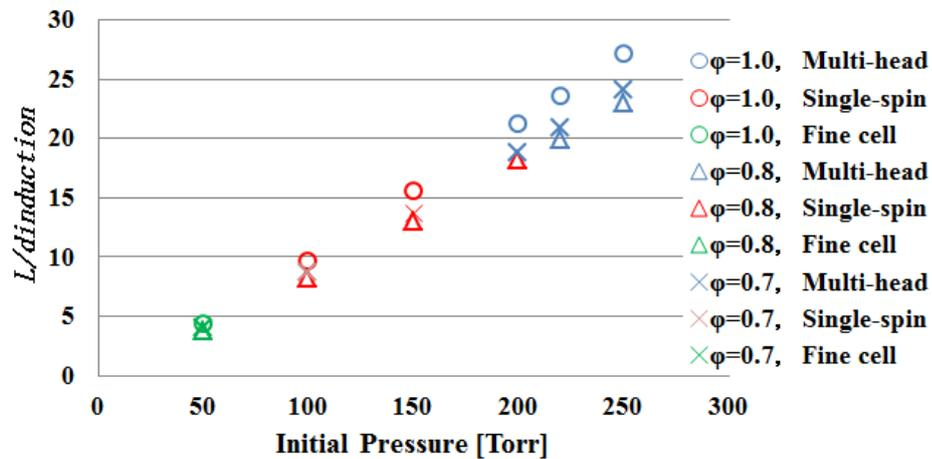
Figure 6. The ratio of the induction length to the circumference.
