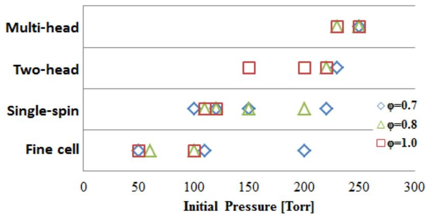
Figure 5. Classification of the soot patterns for various pressures and equivalence ratios.
