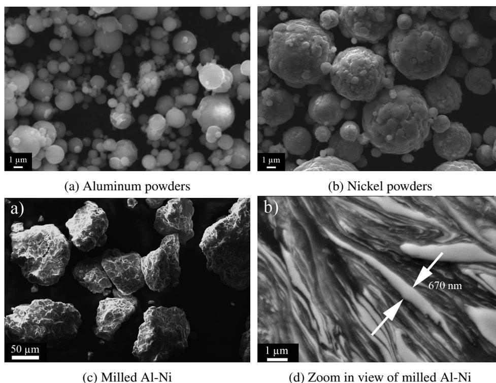
Figure 1: Scanning electron micrograph of the structure of the Al-Ni [5]
