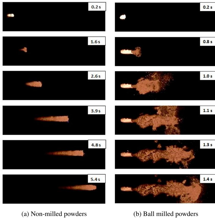
Figure 4: Sequential flames illustrating the flame propagation in Al-Ni system in the 0.75 cm channel width
