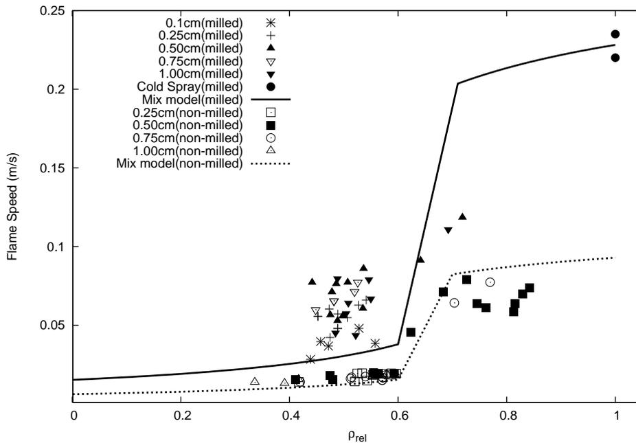
Figure 5: Measured flame speeds in milled and non-milled Al-Ni as function of relative density and comparison with improved Makino's model
