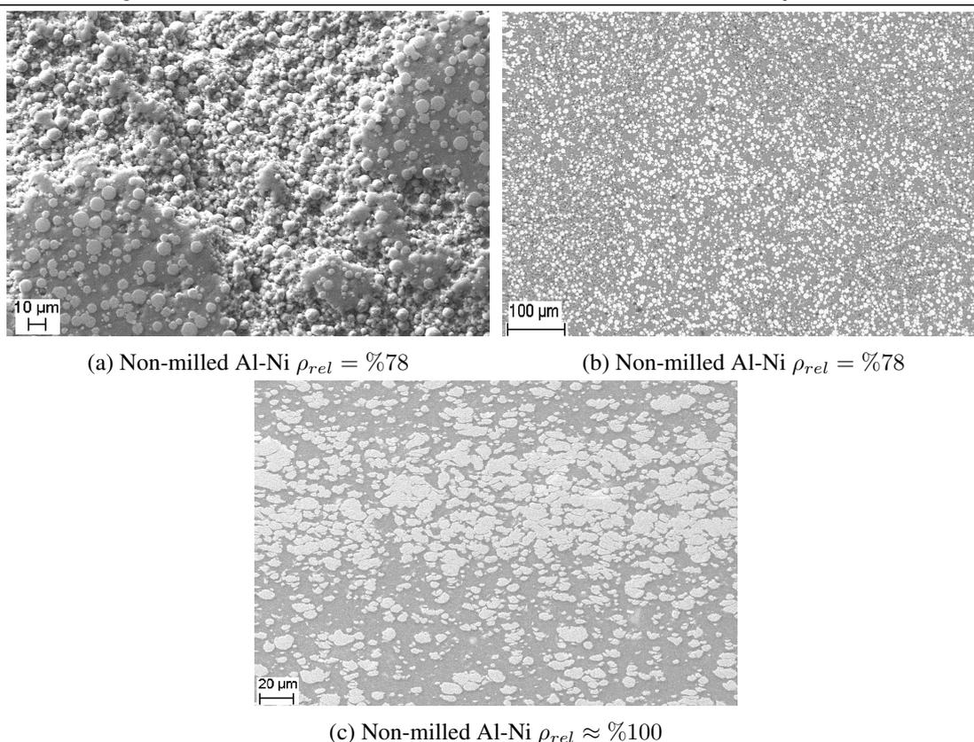
Figure 2: Scanning electron micrograph of the structure of the Al-Ni at different density ratios
