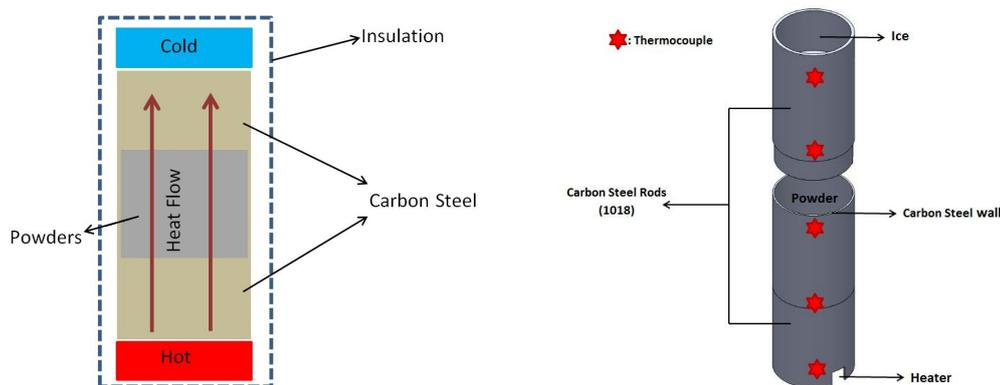
Figure 3: Experimental set-up used to measure the thermal conductivity
