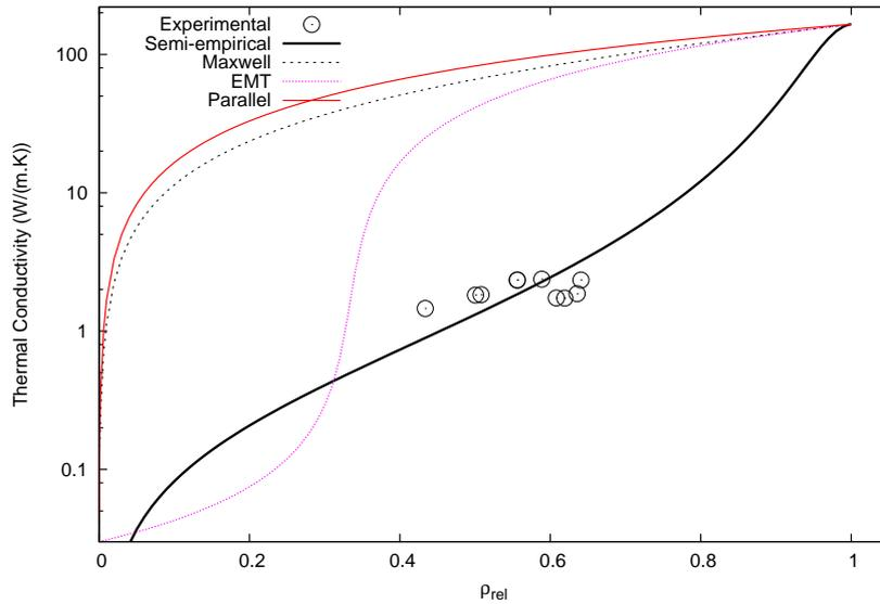
Figure 6: Measured thermal conductivity of Al-Ni powders and comparison with different theoretical models
