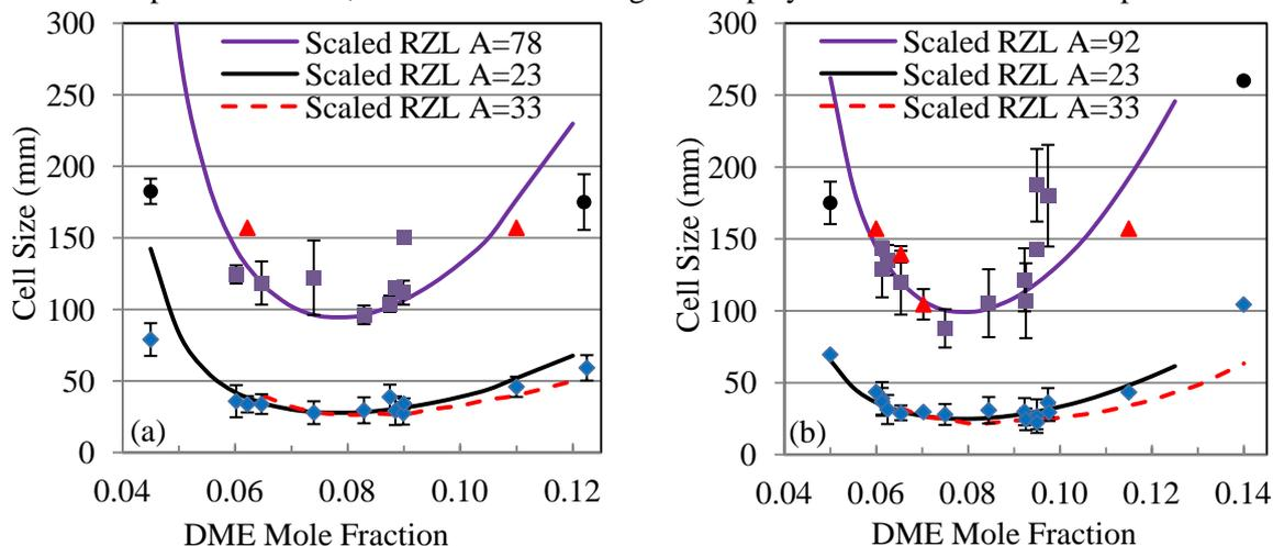
Figure 7. Measured cell size and scaled reaction zone length for DME-air at a) 298K and b) 373K. Small cells -  $\blacklozenge$ ; large cells: orifice plate -  $\blacksquare$ , 0.2 second gas driver -  $\blacktriangle$ , 0.5 second gas driver -  $\bullet$
