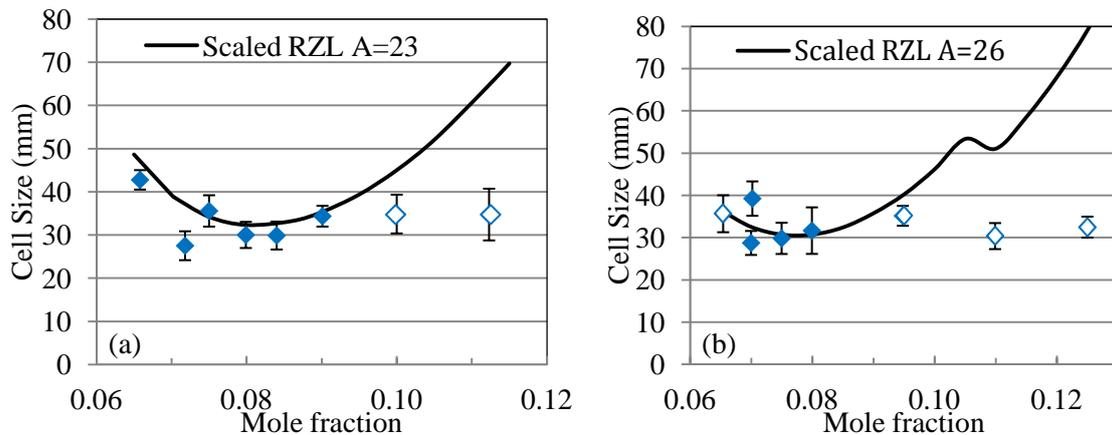
Figure 8. Experimental cell size and scaled reaction zone length for ethanol-air at a) 303/310K and b) 373K. Closed symbol – orifice plates, open symbol – 0.2 second gas driver
