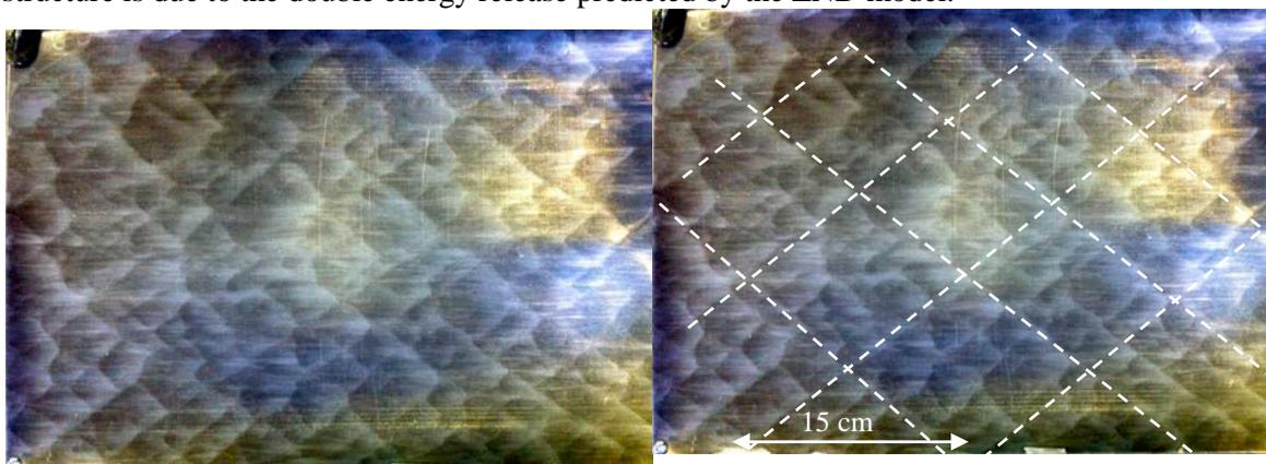
Figure 6. Soot foil for 6.5% DME at 298K showing dominant triple-point trajectories
