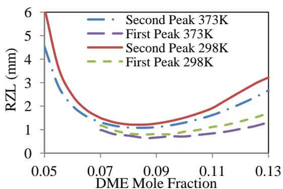
Figure 4. Calculated ZND reaction zone length (RZL) for DME-air mixtures at 298K and 373K
