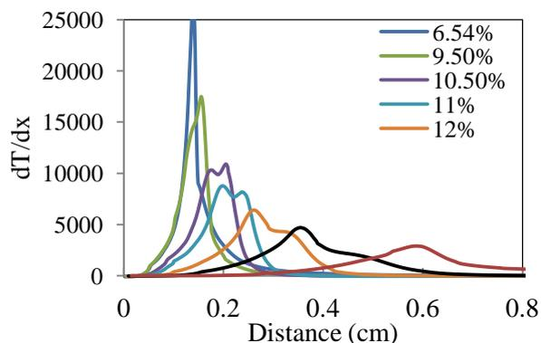
Figure 5. ZND temperature gradient within reaction zone for ethanol-air at 373K for rich mixtures.
