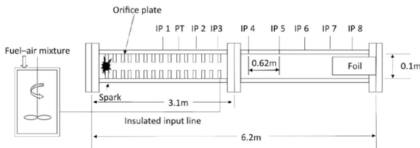
Figure 1. Schematic showing the mixing chamber and orifice plate laden detonation tube.
