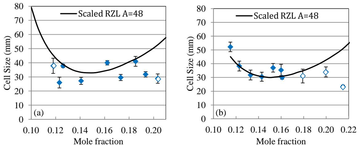
Figure 9. Measured cell size and scaled reaction zone length for methanol-air at a) 303/310K and b) 373K. Closed symbol – orifice plates, open symbol – 0.2 second gas driver
