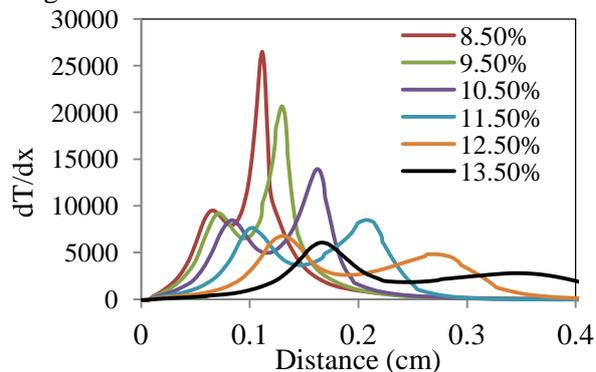
Figure 3. ZND temperature gradient within the reaction zone for DME-air at 373K
