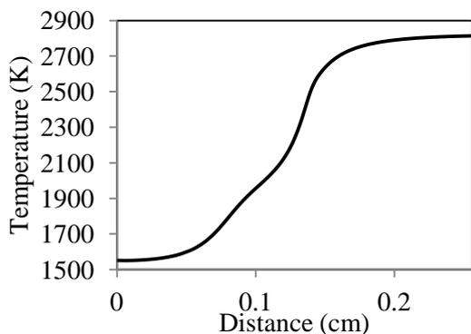
Figure 2. Temperature within ZND detonation reaction zone for 9.0% DME at 298K.
