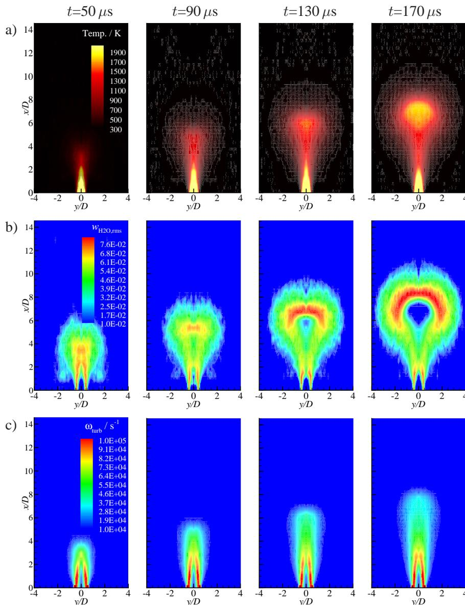
Figure 2: Imaging of ignition event. a) Mean temperature. b) RMS of mass fraction fluctuation of  $\text{H}_2\text{O}$ ,  $w_{\text{H}_2\text{O},\text{rms}}$ . c) Turbulence frequency.
