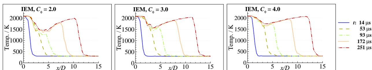
Figure 3: Mean temperature along the centreline at different times for simulations with various  $C_\phi$ .
