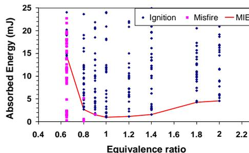
Figure 7. Laser ignition diagram for gaseous n-decane – air mixtures at 347 K and P = 1 bar.
