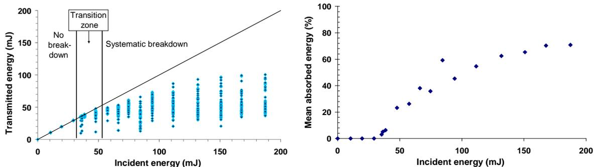
Figure 2. Laser breakdown data obtained with a n-C<sub>10</sub>H<sub>22</sub> – N<sub>2</sub> mixture ( $P_0 = 1$  bar,  $PC_{10}H_{22} = 26$  mbar,  $T_0 = 347$  K). Left: Transmitted energy versus incident energy. Right: Mean absorbed energy versus incident energy.
