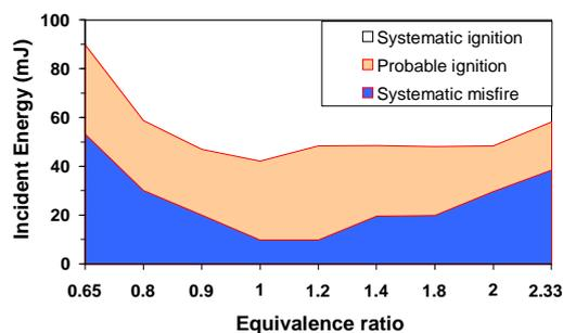
Figure 6. Ignition domains with respect to fuel equivalence ratio and incident energy for gaseous n-decane – air mixtures at 347 K and P = 1 bar.
