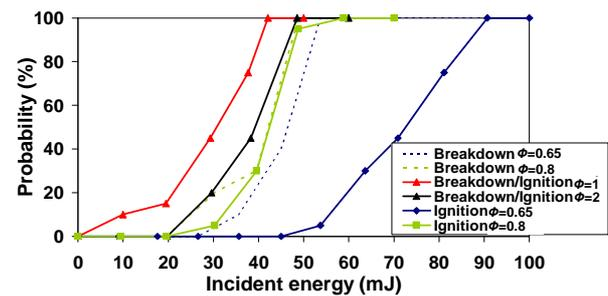
Figure 5. Ignition and breakdown probabilities of different n-decane – air mixtures.
