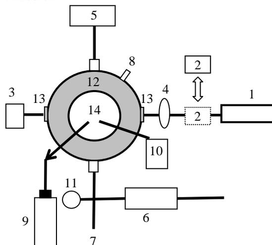
Figure 1. Sketch of the experimental apparatus (1) Nd:YAG laser (2) mobile energy meter (3) fixed energy meter (4) 150 mm focal length lens (5) pressure transducer (6) vacuum pump (7) gas inlet (8) septum (9) camera (10) photodiode detector (11) manometer (12) combustion chamber (13) antireflection-coated window (14) quartz window.
