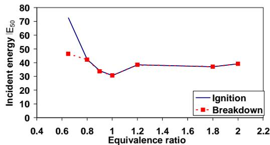
Figure 4. Evolution of  $E_{50}$  based on incident energy for different n-decane – air mixtures.
