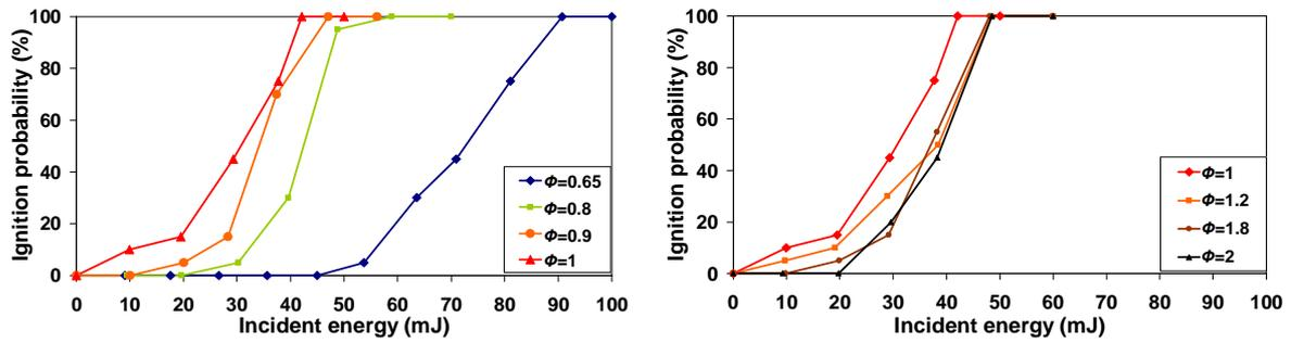
Figure 3: Ignition probabilities for lean (left) and rich (right) n-decane – air mixtures.
