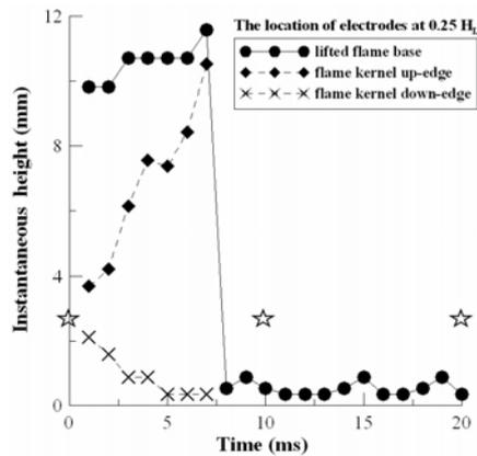
Figure 4. The sequential instantaneous location of lifted flame bases and the flame-kernel edges propagating from the discharge location of  $0.25 H_L$  to the downstream lifted flame base and to the upstream tube exit as using a repetitive discharge rate of 100 Hz for a jet exit velocity of 8.6 m/s, star symbols represent the pulsed-arc discharges for a repetitive rate at 100 Hz.
