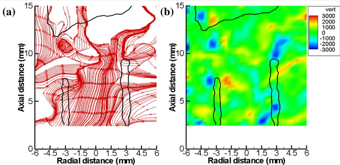
Figure 5. The flow-field of a successful flame-kernel initiated by pulsed-arc discharge with the contours of flame kernels and lifted flame base measured by PIV. (a) Instantaneous velocity streamlines profile. (b) Vorticity field profile.
