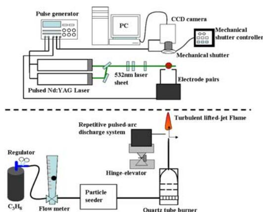
Figure 1. Schematic diagram of the experimental setup.
