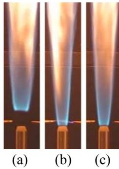
Figure 3. Observation of repetitive pulsed-arc-enhanced flame reattachment phenomena for jet exit velocity of 8.6 m/s. (a) Without discharge. (b) With discharge. (c) Discharge ceased.
