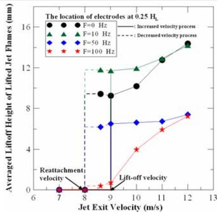
Figure 2. Averaged liftoff height versus jet exit velocity for different repetitive rates as the electrode location of  $0.25 H_L$ , dashed lines: hysteresis region, solid lines: liftoff region.
