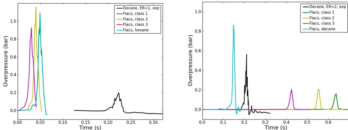
Figure 2: Overpressure as a function of time for the geometry with two baffles. On the left, decane with ER=1. On the right, decane with ER=2. The black graphs represent experimental results.
