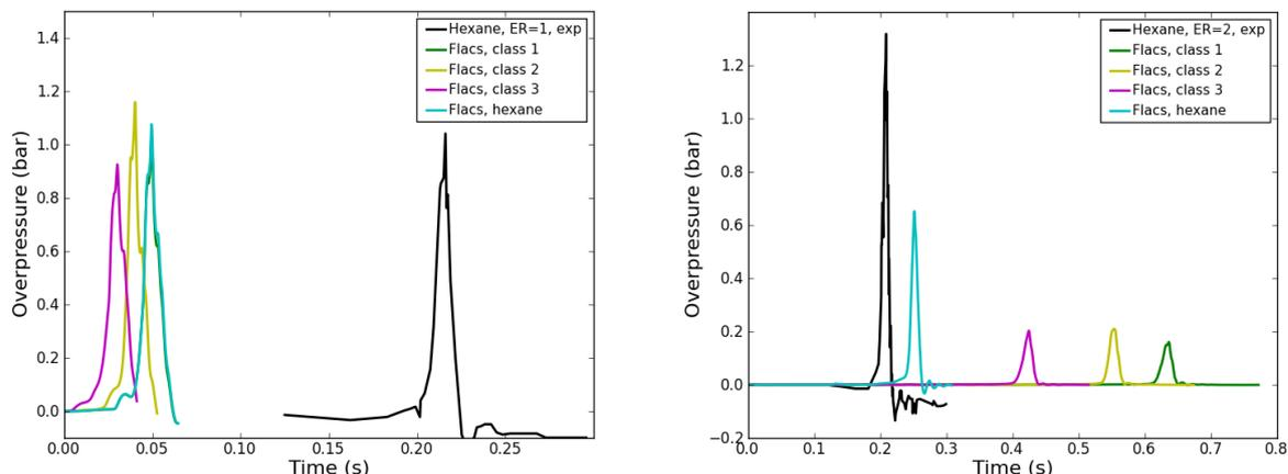
Figure 4: Overpressure as a function of time for the geometry with two baffles. On the left, hexane with ER=1. On the right, hexane with ER=2.
