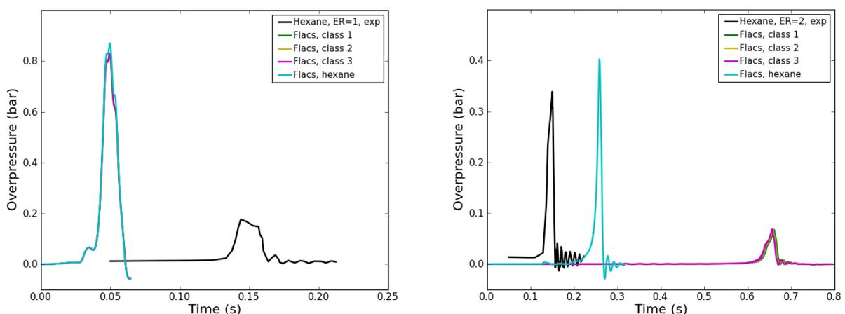
Figure 3: Overpressure as a function of time for the geometry with one baffle. On the left, hexane with ER=1. On the right, hexane with ER=2.
