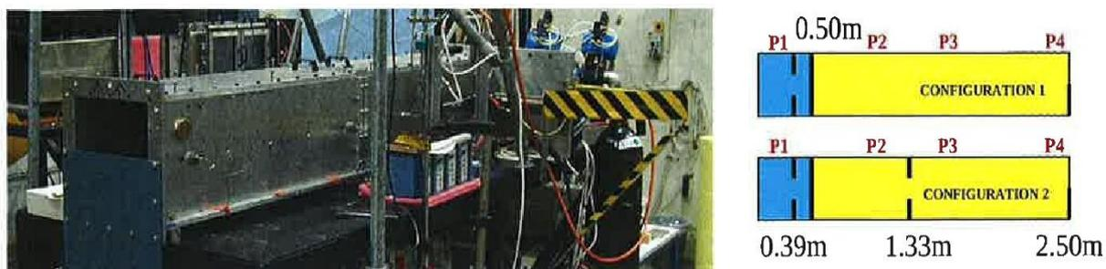
Figure 1. Test rig with baffles configurations on the right. Blue section represents the lean propane, the yellow one the oil mists from sprays.
