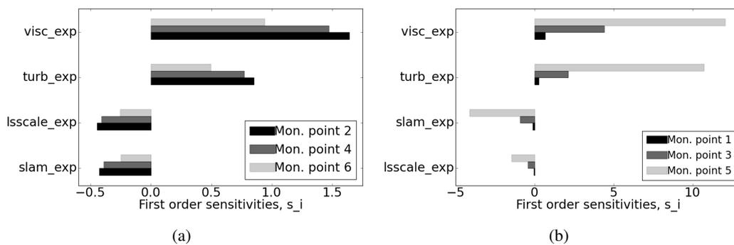
Figure 2: First order sensitivity analysis of the maximum overpressure to a selection of empirical parameters, obtained in two monitor points for the MERGE B (a) and HSE Beta (b) configurations.
