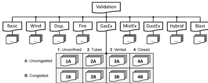
Figure 1: A classification scheme for the GasEx application of FLACS [7].
