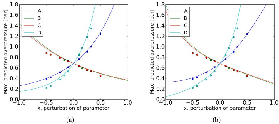
Figure 3: Model (dots) and response surface (lines) for (a) a second order logarithmic surface and (b) a partial third order logarithmic surface, legend labels defined according to Table 1.
