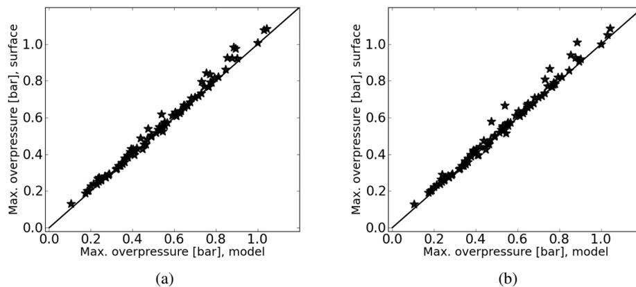
Figure 4: Model and response surface agreement for (a) a second order logarithmic surface and (b) a partial third order logarithmic surface.
