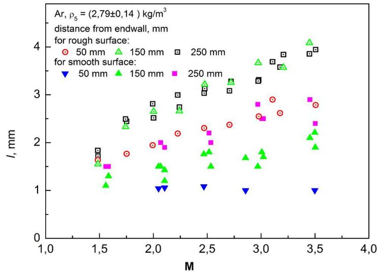
Figure 3. Length  $l$  vs. Mach number of an incident shock wave for argon.
