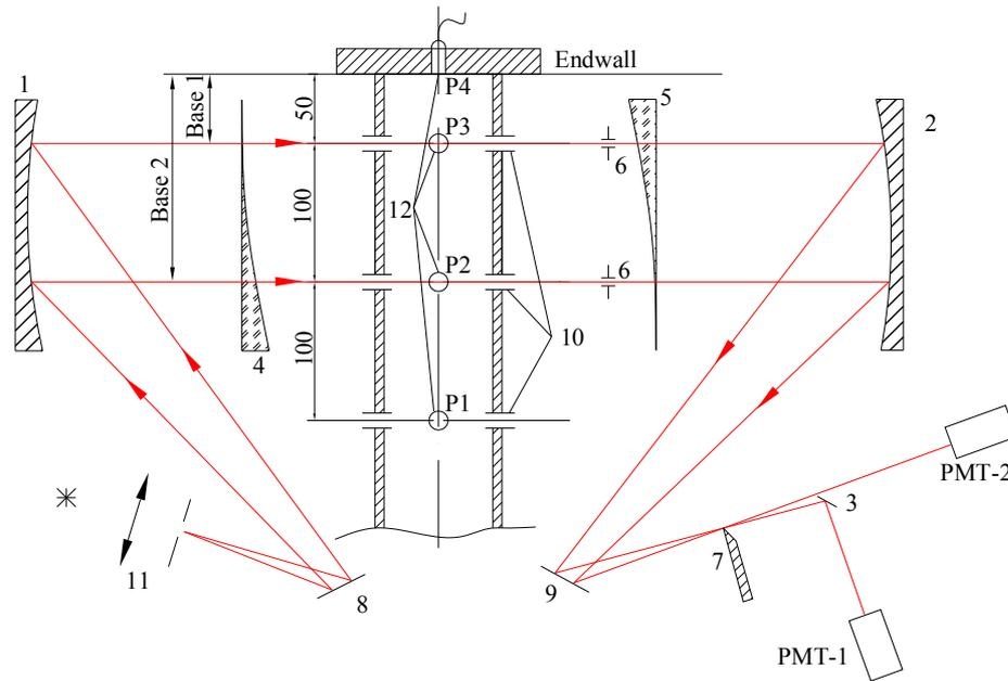
Figure 2. Optical scheme, the scheme of light beams propagations, and the arrangement of pressure sensors: 1, 2, 3 – mirrors; 4, 5 – menisci; 6 – vertical slot 0.55 mm in width; 7 – knife edge; 8, 9 – rotary elements of the setup; 10 – optical windows; 11 – vertical slot and the lighting system of IAB-451; 12 – pressure sensors.
