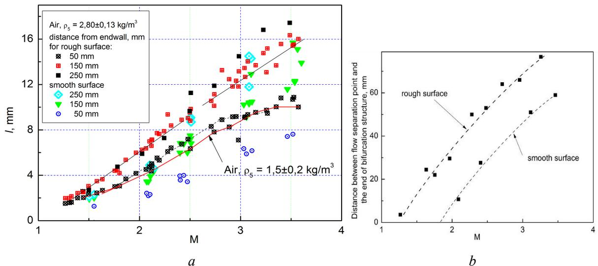
Figure 5. Bifurcation characteristic size vs. Mach number of an incident shock wave for air: a)  $l$  vs. Mach number of an incident shock wave; b) distance between the flow separation point and the end of bifurcation structure at 50 mm to the endwall.
