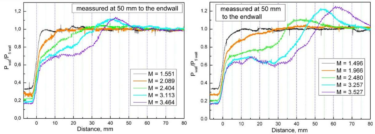
Figure 4. Surface pressure distribution measured at 50 mm to the endwall. Left: smooth surface. Right: rough surface.
