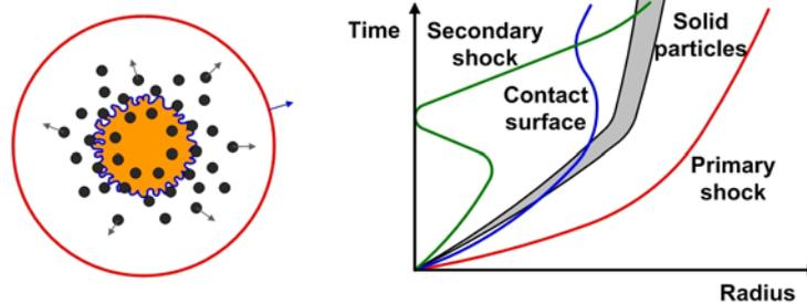
Figure 1. Wave diagram of typical explosives with solid particles.
