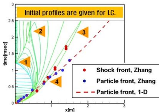
Figure 3. NM explosion with 463μm steel particles: 1 secondary shock reflection point; 2 interaction of secondary shock with contact surface; 3 primary shock wave; 4 overtaking point of shock by particle front.
