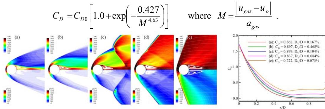
Figure 2. Drag coefficient estimation of sphere in detonation flow fields: (a)  $C_D=0.862$ ; (b)  $C_D=0.897$ ; (c)  $C_D=0.899$ ; (d)  $C_D=0.837$ ; (e)  $C_D=0.722$ . [5]
