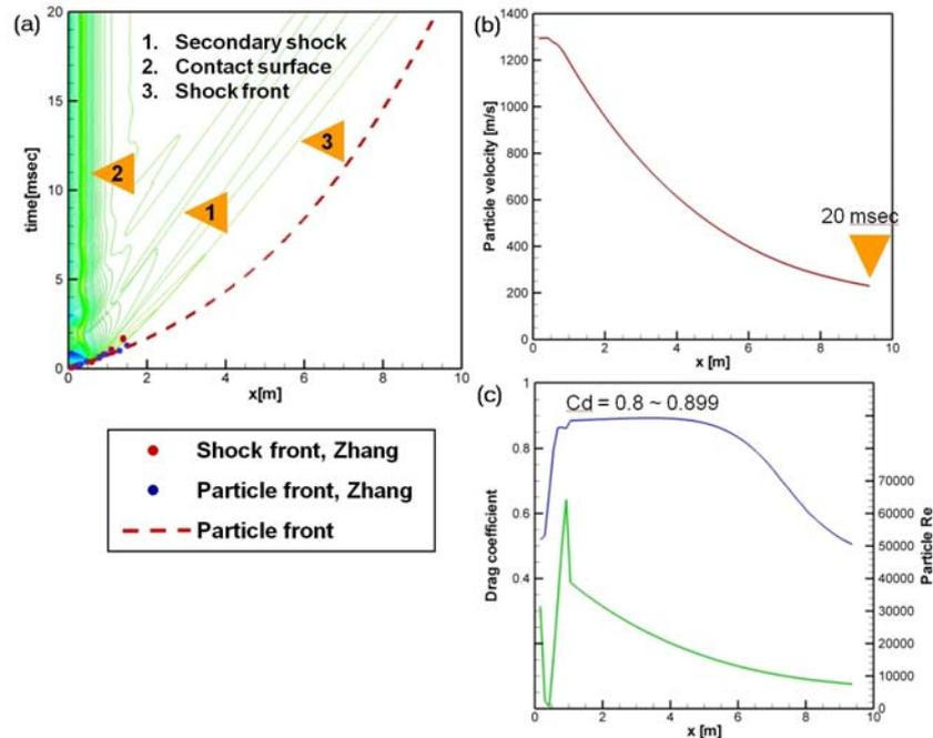
Figure 4. Particle velocity and drag coefficient variations: (a) wave diagram; (b) particle front velocity; (c) drag coefficient (upper blue line) and particle Reynolds number (lower green line).
