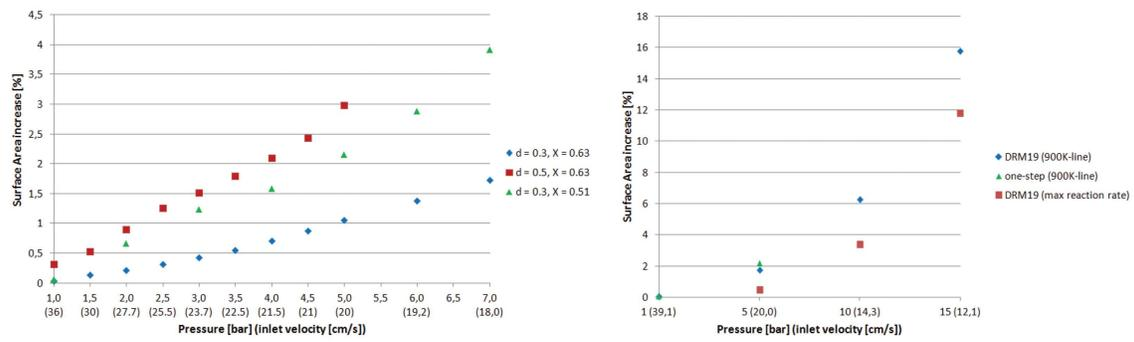
Figure 3: Surface increase of the flame
