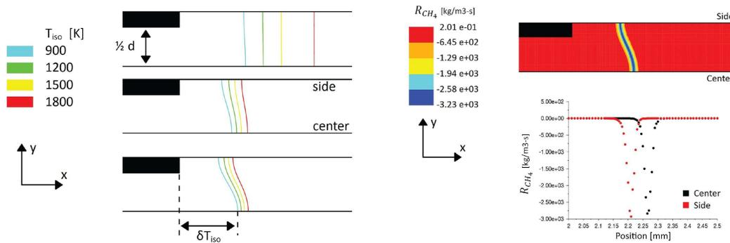
Figure 2: (Left)  $\delta T_{iso}$  for 1, 5 and 10 bar (top to bottom) (Right) Net reaction rate of methane at 10 bar
