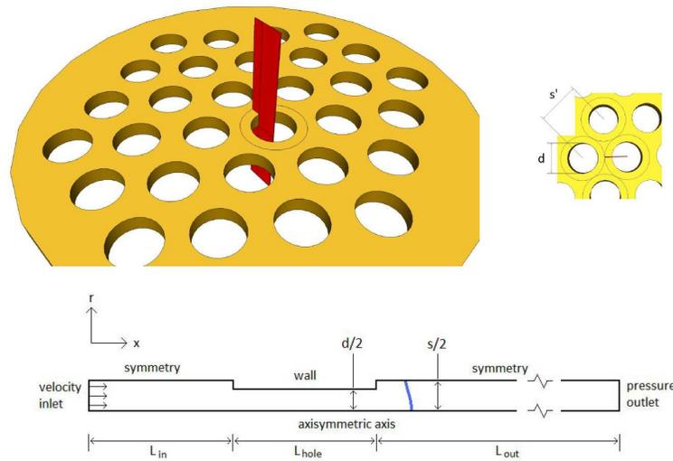
Figure 1: (Top) Axisymmetric domain (Bottom) Computational domain
