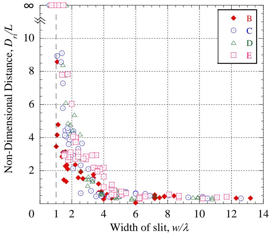
Figure 6. Relationship between non-dimensional re-initiation distance  $D_{ri}/L$  and non-dimensional slit width  $w/\lambda$ .
