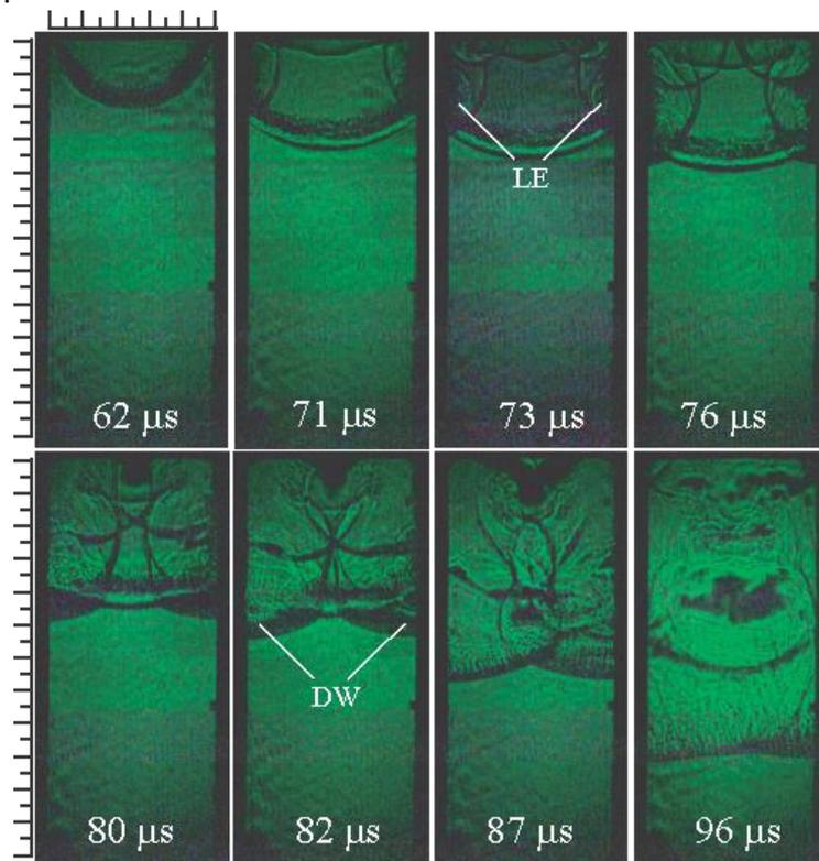
Figure 3. Schlieren photographs ( $2\text{H}_2 + \text{O}_2$ ,  $p_0 = 50$  kPa, Type A,  $w = 15$  mm).
