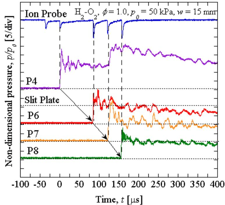
Figure 4. Pressure histories ( $2\text{H}_2 + \text{O}_2$ ,  $p_0 = 50$  kPa, Type A,  $w = 15$  mm).
