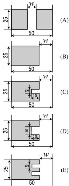
Figure 2. Configuration of the slit-plate.
