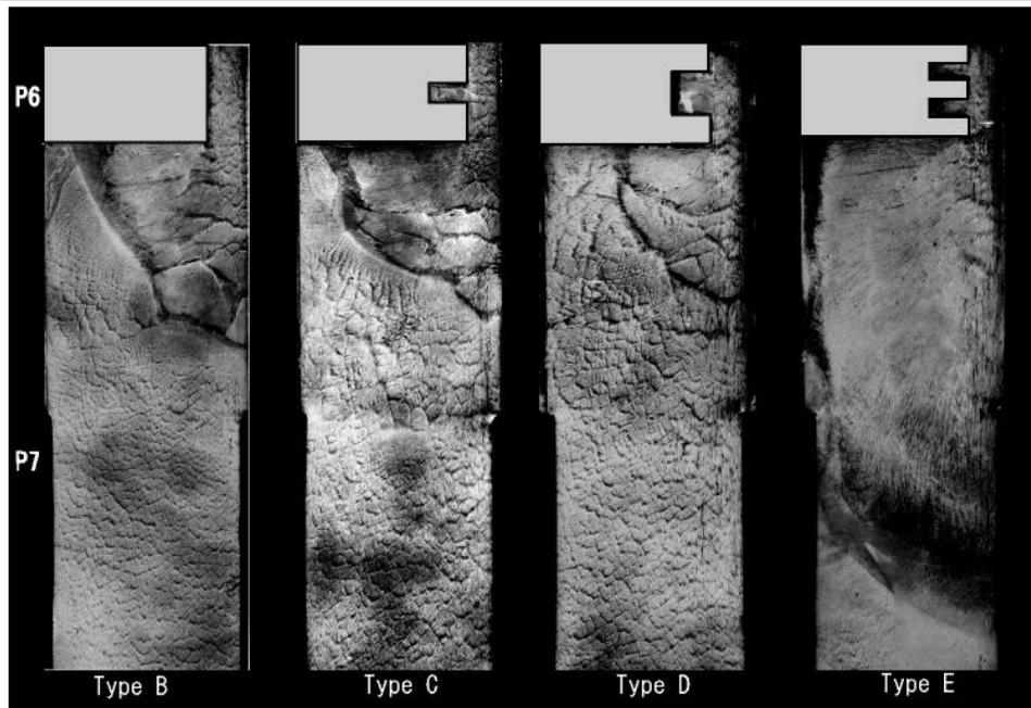
Figure 5. Soot-track record for Type B, C, D and E ( $2\text{H}_2 + \text{O}_2$ ,  $p_0 = 60 \text{ kPa}$ ,  $w = 8 \text{ mm}$ ).
