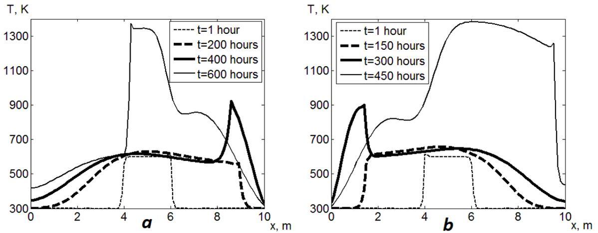
Figure 3. Distribution of the solid medium temperature in the porous object with gravity field and without the pressure difference at object boundaries (a), in the object with the pressure difference at object boundaries and without gravity field (b)
