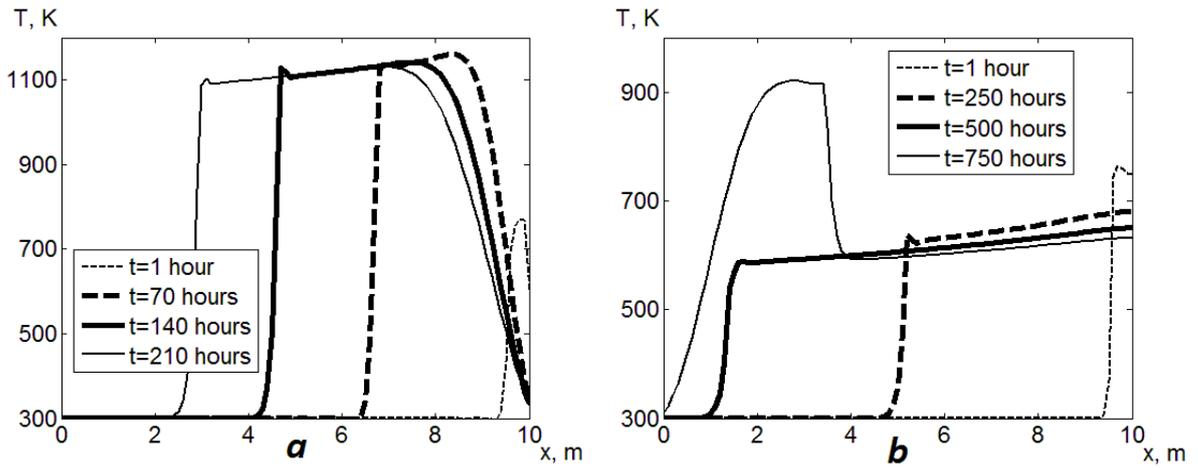
Figure 2. Distribution of the solid medium temperature in the porous object with gravity field and without the pressure difference at object boundaries (a), in the object with the pressure difference at object boundaries and without gravity field (b)
