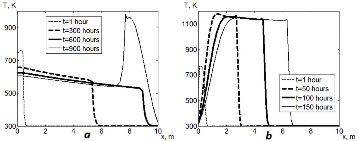
Figure 1. Distribution of the solid medium temperature in the porous object with gravity field and without the pressure difference at object boundaries (a), in the object with the pressure difference at object boundaries and without gravity field (b)
