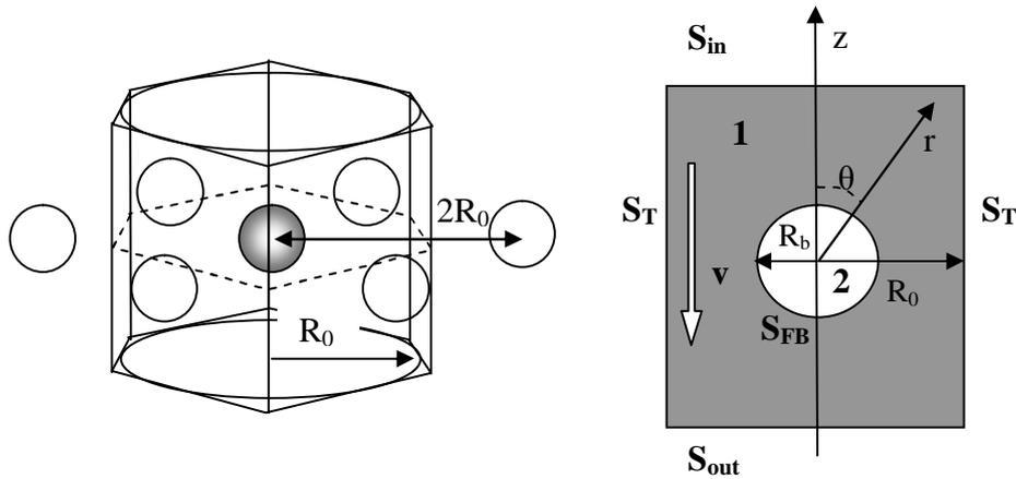
Figure 1. Left: Scheme of flame balls planar hexagonal array. Right: Scheme of flame ball propagating with velocity  $v$  in tube with radius  $R_0$ . (Shaded region is unburned mixture).
