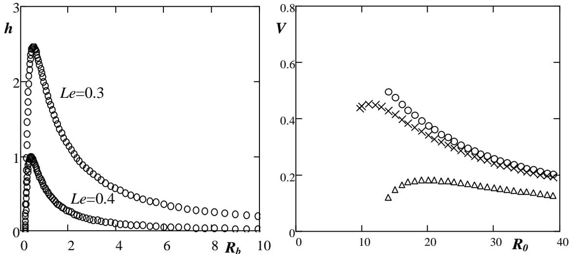
Figure 2. Left: Heat loss  $h$  dependencies on flame radius  $R_b$ , evaluated at  $N=10$ ,  $\sigma = 0.2$ , Right: Dependencies of flame ball propagation velocity  $v$  on tube radius  $R_0$ , evaluated at  $Le=0.3$ ,  $h=0.3$  (circles),  $Le=0.3$ ,  $h=0.5$  (crests) and  $Le=0.4$ ,  $h=0.3$  (triangles).
