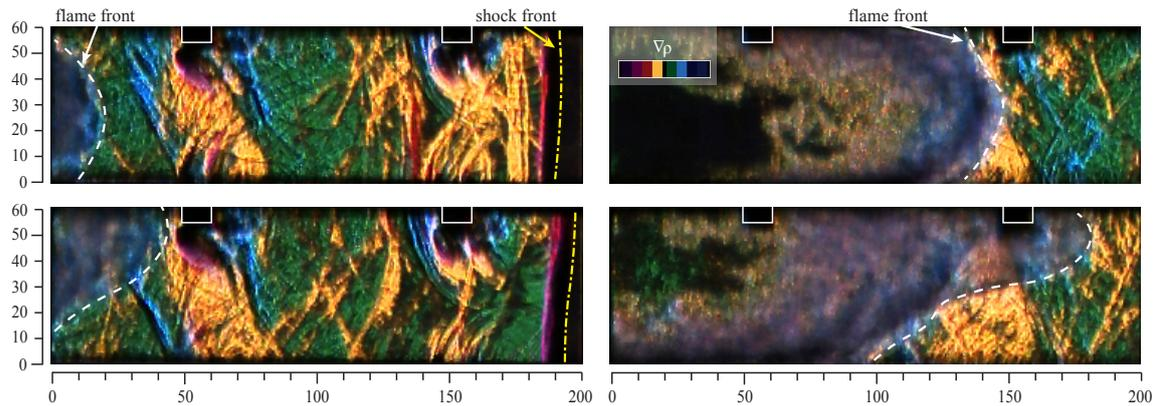
Figure 2: Color schlieren images showing shock waves and flame front in 15 %vol  $H_2$ -air mixture propagating in the unobstructed part of the channel; First row: homogeneous mixture at two different stages; Second row: inhomogeneous mixture with steep concentration gradient ( $t_d = 3$  s) at two different stages.
