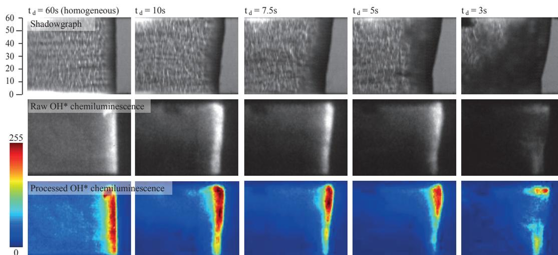
Figure 4: Shadowgraph and OH\* chemiluminescence images of detonations in 30 %vol H<sub>2</sub>-air mixture with different concentration gradients.
