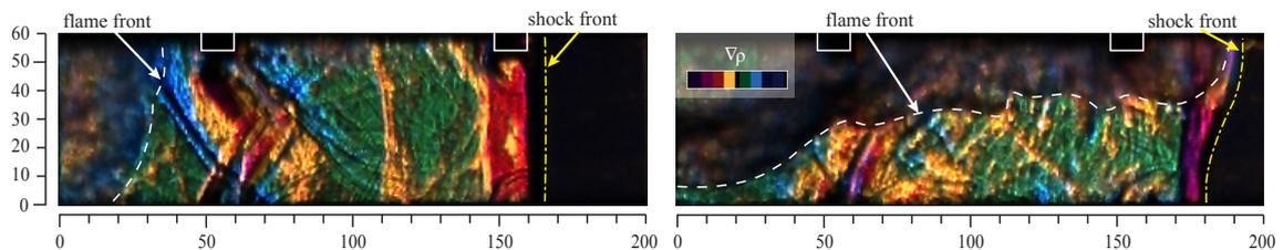
Figure 3: Color schlieren images showing shock waves and flame front in 20 %vol  $H_2$ -air mixture propagating in the unobstructed part of the channel; Left: homogeneous mixture; Right: inhomogeneous mixture with steep concentration gradient ( $t_d = 3$  s).
