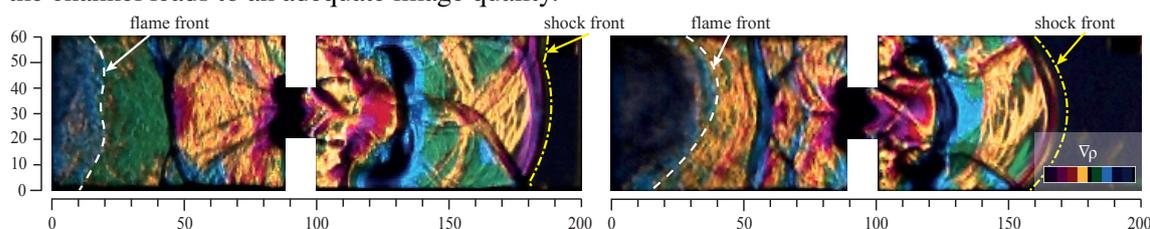
Figure 1: Color schlieren images showing shock waves and flame front in 15 %vol H<sub>2</sub>-air mixture in the BR60S300 obstacle configuration; Left: homogeneous mixture; Right: inhomogeneous mixture with steep concentration gradient ( $t_d = 3$  s).
