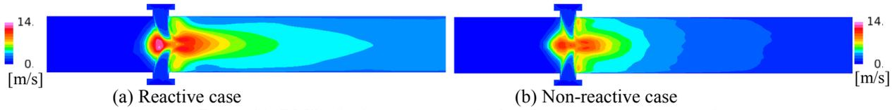
Figure 11. RMS of velocity magnitude distribution fluctuation (xy plane)
