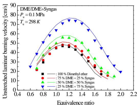
Figure 4 Measured (symbol) and predicted (line) unstretched laminar burning velocities in DME/DME+Syngas flames at  $P_u = 0.1$  MPa and  $T_u = 298 \pm 3$  K.
