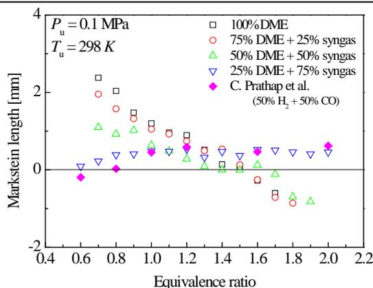
Figure 2 The effect of syngas addition on the Markstein length in DME-air premixed flames;  $P_u = 0.1$  MPa and  $T_u = 298 \pm 3$  K.
