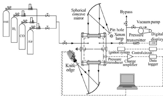
Figure 1 Schematic representation of the experimental setup.
