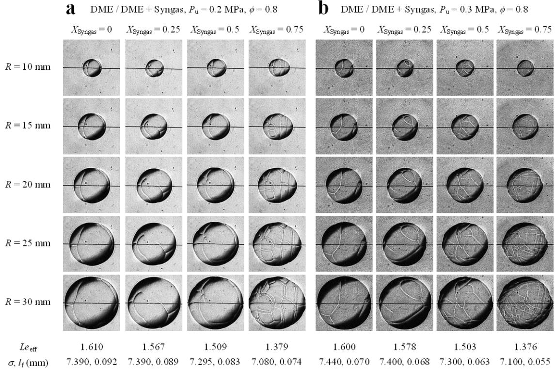
Figure 5 Syngas effects on cellular instability of DME-air premixed flames at  $P_u = 0.2$  MPa (a),  $0.3$  MPa (b),  $T_u = 298 \pm 3$  K, and  $\phi = 0.8$ .
