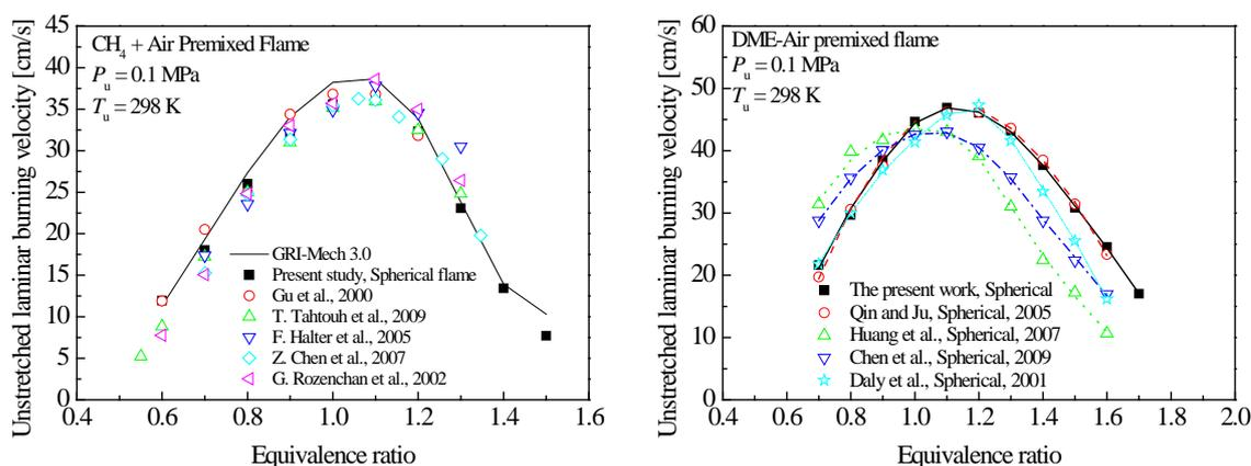
Figure 3 Unstretched laminar burning velocities measured at  $P_u = 0.1$  MPa and  $T_u = 298 \pm 3$  K in  $\text{CH}_4$ -air (left) and DME-air (right) premixed flames.
