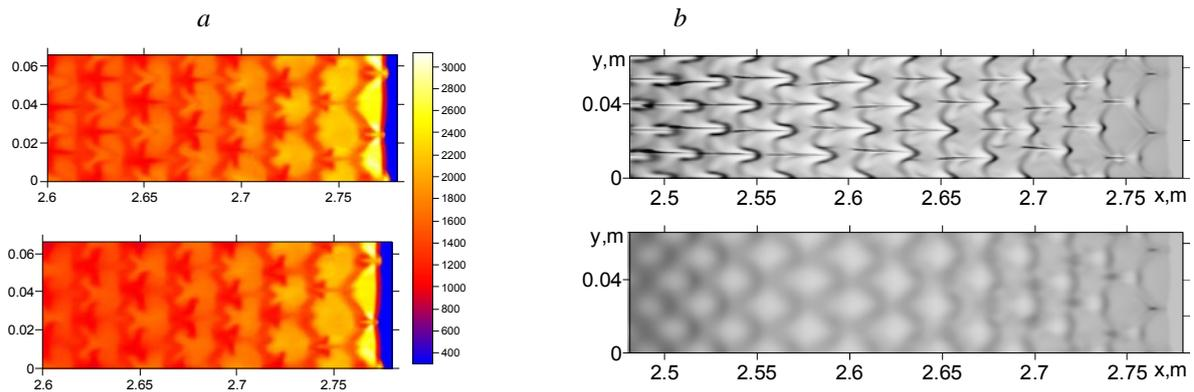
Figure 4. Cellular detonations in aluminum suspensions in gas with inert particles, gas temperature field (a); inert particles density field (b): comparison of results [2] (top) and collisional model (bottom,  $e_{c0} = 0.0001 \text{ m}^2/\text{ms}^2$ ).
