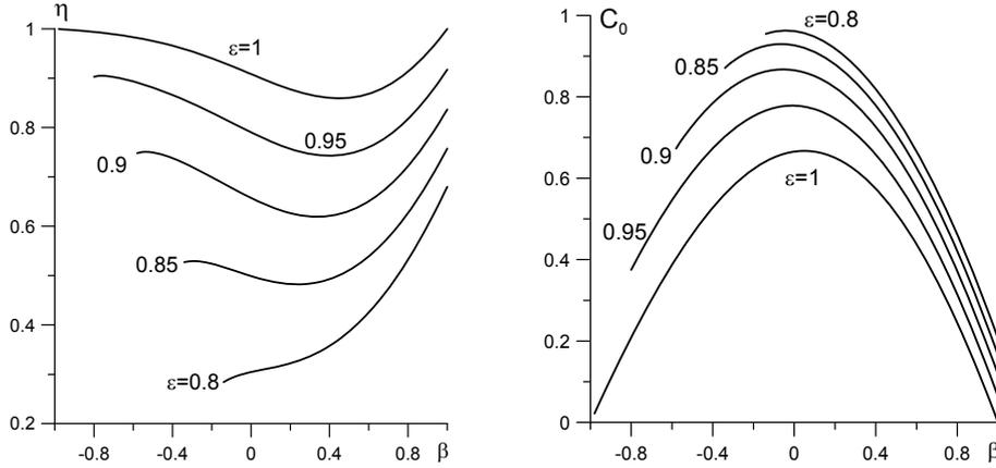
Figure 1. Dependence of the parameters  $\eta$  and  $C_0$  on the restitution and roughness coefficients
