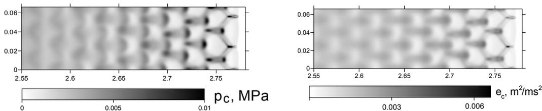
Figure 5. Cellular detonations in aluminum suspensions in gas with inert particles: collisional pressure (a) and chaotic energy distributions (b) at  $e_{c0} = 0$ ,  $\eta = 1$ .
