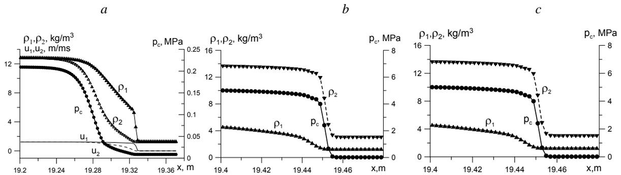
Figure 3. Stationary SW structures at  $M_0 = 5$ ,  $e_{c0} = 0.01$  m<sup>2</sup>/ms<sup>2</sup>: type I,  $d=10$   $\mu$ m,  $\xi_0 = 0.5$  (a); type II,  $d=20$   $\mu$ m,  $\xi_0 = 0.7$  (b)
