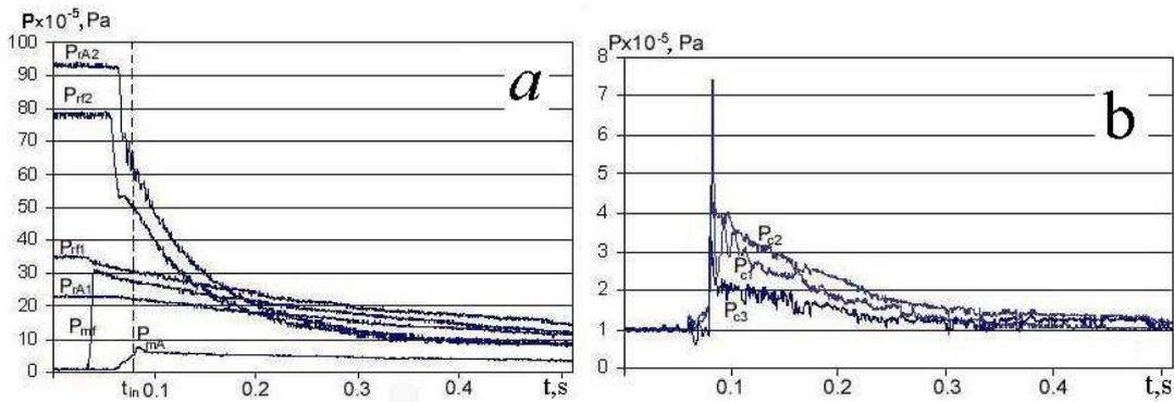
Figure 2. Oscillograms of pressures in the receivers and manifolds (a) and in the combustor (b).
