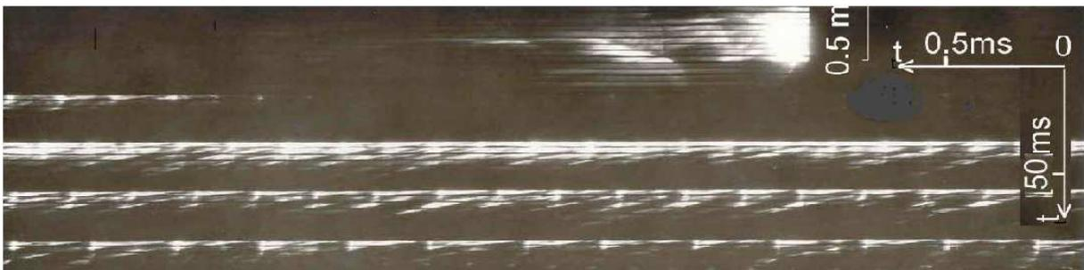
Figure 3. Photographic records with the beginning of the transitional process and further development of continuous spin detonation in the combustor.
