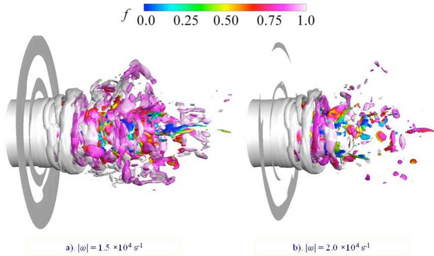
Figure 3. Snapshots of vorticity magnitude iso-surface colored by the mixture fraction. Pressure is set to 10 MPa,  $T_{\text{LOX}}=120$  K,  $T_{\text{CH}_4}=300$ K. Injector dimension:  $D_{\text{LOX}}=3.42$  mm, LOX post  $\delta=0.38$  mm,  $D_{\text{CH}_4}=5.18$  mm.
