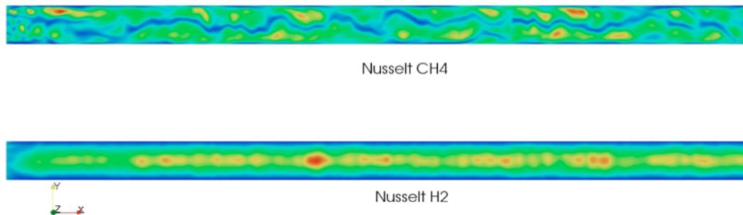
Figure 1. CH<sub>4</sub> and H<sub>2</sub> Nusselt number using the original code (4CD).
