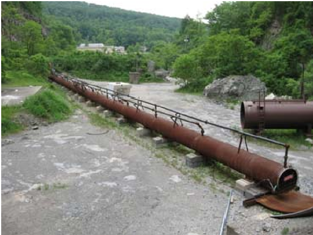
Figure 1 - Overview of the gas explosion test facility (GETF) for large-scale, methane-air detonation and DDT experiments at NIOSH Lake Lynn Laboratory.
