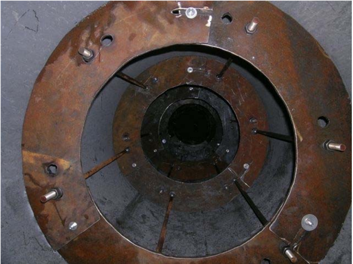
Figure 3 – Baffles with blockage ratio BR = 0.6 and spacing S=d=105 cm installed in the tube.
