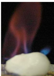
Figure 6. The Spherical methane burn after approximately 5 seconds
