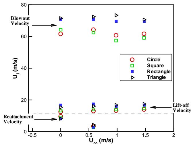
Figure 3. Comparison of the flame lift-off, blowout and reattachment velocities for different nozzles at different co-airflow exit velocities.
