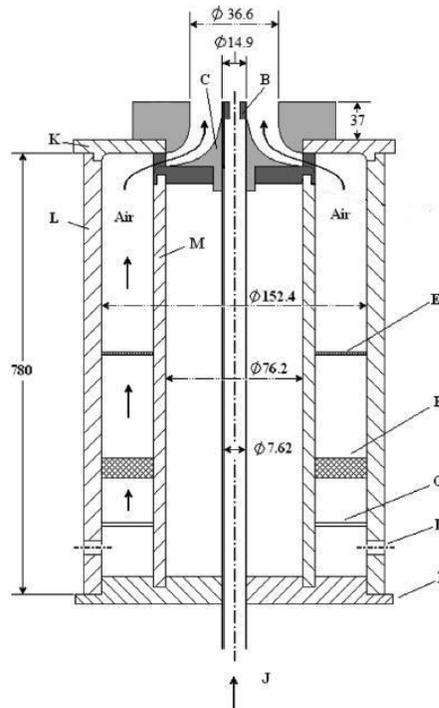
Figure 1. Schematic of the experimental burner set-up: B=nozzle, C=nozzle holder, E=fine screen, F=honeycomb, G=coarse screen, H=four equally spaced tangential air ports, I=bottom plate, J=methane gas flow, K=top plate, L=outer chamber, M=inner chamber [3].
