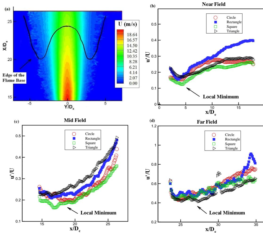
Figure 4. PIV measurements of the reacting jet. (a) a typical velocity contours for the lifted flame which also shows the flame base, and the  $u'/U$  profiles for (b) the flame base stabilized in the near-field ( $U_j = 12$  m/s), (c) the flame base stabilized in the mid-field ( $U_j = 18$  m/s), and (d) the flame base stabilized in the far-field ( $U_j = 24$  m/s).
