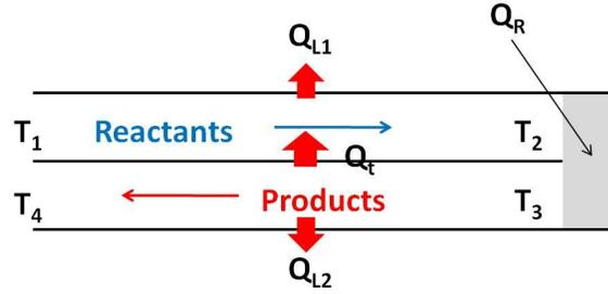
Figure 2. Schematic diagram of counter-current heat recirculating combustor.
