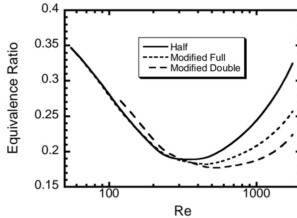
Figure 4. Extinction limits vs. Re for different scale combustors with modified  $\alpha$ .
