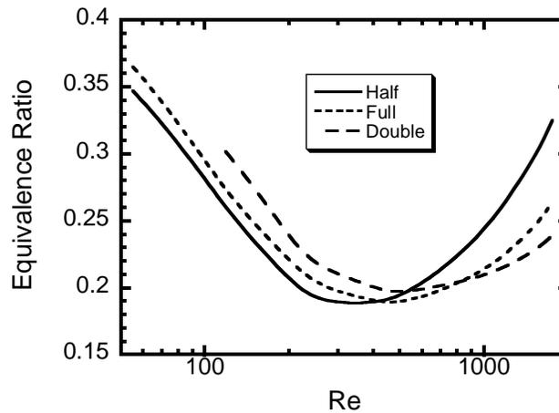
Figure 3. Extinction limits vs. Re for different scale combustors.
