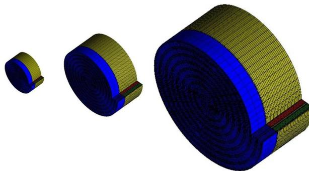
Figure 1. 3 different-scale but geometrically identical 3D numerical model of Swiss-roll combustors (Half, Full, and Double).
