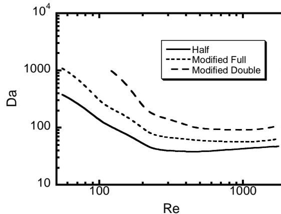
Figure 6. Da at limits vs. Re for different scale combustors (with the modified  $\alpha$ ).
