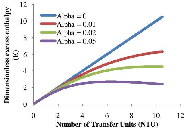
Figure 5. Dimensionless excess enthalpy vs. NTU for different  $\alpha$ .
