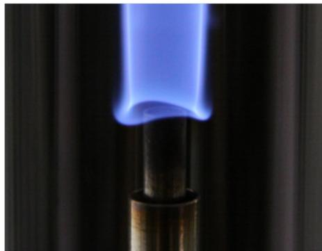
Fig. 2. Direct photograph of the diffusion flame base. The conditions are  $\Delta z = 12$  mm,  $U_f = 300$  cm/s,  $U_p = 20$  cm/s ( $L_p = 7.068$  cm<sup>3</sup>/s),  $U_a = 10$  cm/s and  $D_{outer} = 10$  mm.
