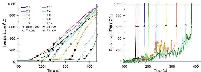
Figure 2. Temperatures (left) and time derivatives of temperatures (right) for test number 22: initially turbulent mixture of 6.0 % propane in air, ignited by an electric spark.
