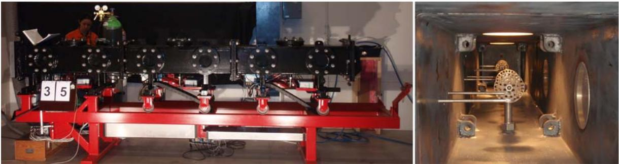
Figure 1. The 3.6 metre flame acceleration tube (left), and internal view of the tube showing flame probes, dispersion nozzles, brackets for fixing obstacles, and windows (right).
