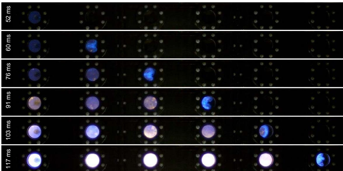
Figure 7. Selected frames from the high-speed video camera for Test 20: 4.5 % propane, initially quiescent.
