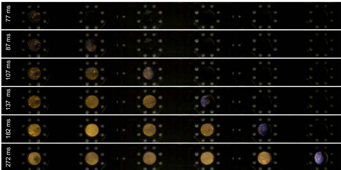
Figure 6. Selected frames from the high-speed video camera for Test 13: 3.0 % propane, initially turbulent.
