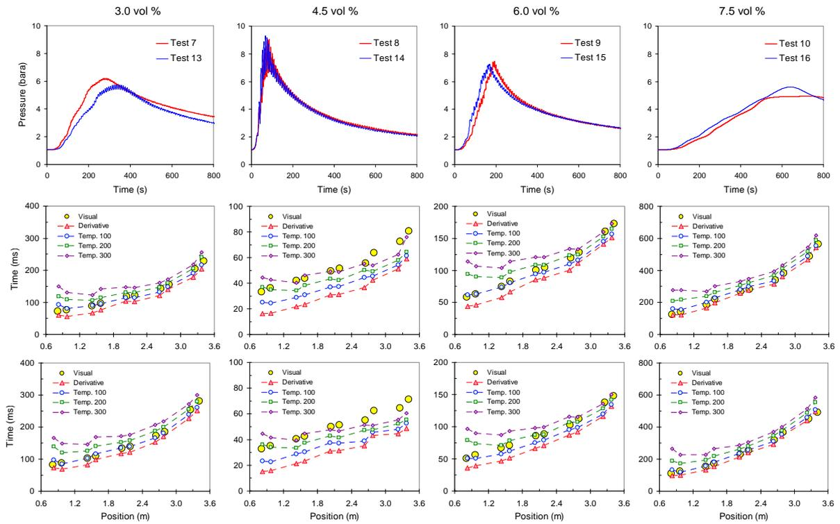
Figure 3. Measured pressure-time histories and estimated flame arrival times for two repeated tests in initially turbulent mixtures of 3.0, 4.5, 6.0 and 7.5 per cent propane in air.
