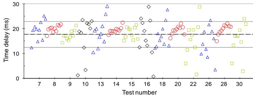
Figure 5. Delay between onset of rapid temperature rise, measured with thermocouples, and visual observation of flame arrival from high-speed video recordings of the experiments with gaseous fuel. The horizontal lines indicate the average value (17.7 ms), plus/minus one standard deviation (5.2 ms).
