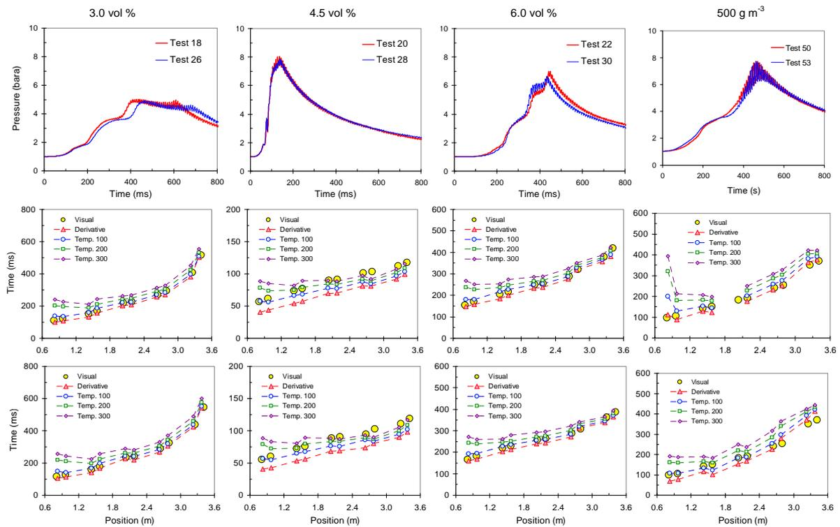
Figure 4. Measured pressure-time histories and estimated flame arrival times for two repeated tests with initially quiescent mixtures of 3.0, 4.5 and 6.0 per cent propane in air, as well as initially turbulent mixtures of 500 g m<sup>-3</sup> maize starch in air.
