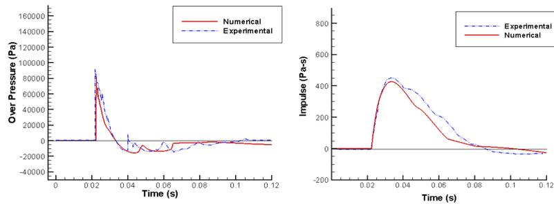
Figure 5. Comparison of the predicted and measured overpressure and impulse for hydrogen-air cloud
