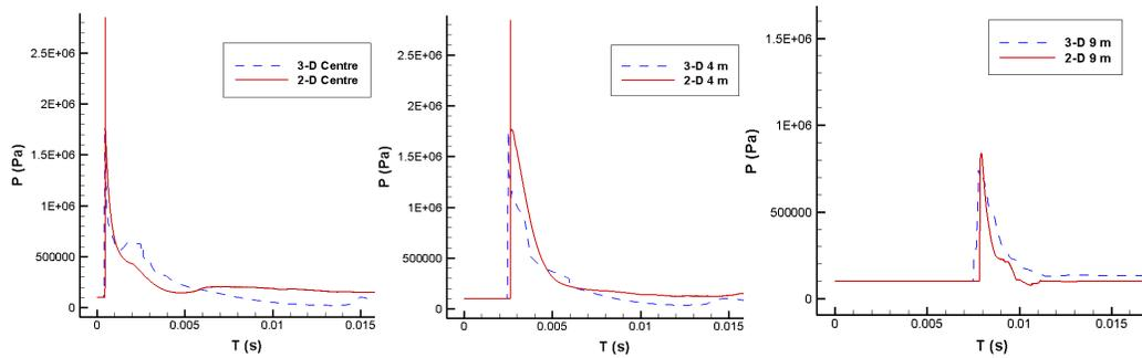
Figure 8. Comparison of pressure vs-time curve (propane-air mixture) at 3 monitoring points between the pancake (solid-red line) and the hemispherical clouds (blue-dashed line)
