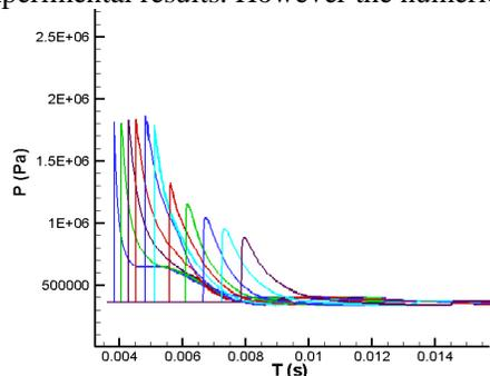
Figure 6. Pressure diagram for propane-air cloud, Pressure drop for hemispherical cloud
