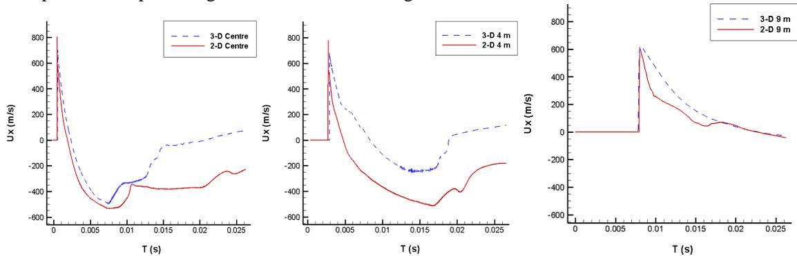
Figure 9. Comparison of the horizontal velocity (propane-air mixture) at 3 monitoring points between the pancake (solid-red line) and the hemispherical clouds (blue-dashed line).
