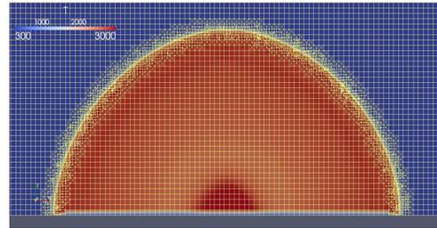
Figure 2. The mesh refinement at the shock front.
