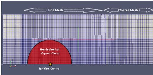
Figure1. The Numerical domain and the Mesh
