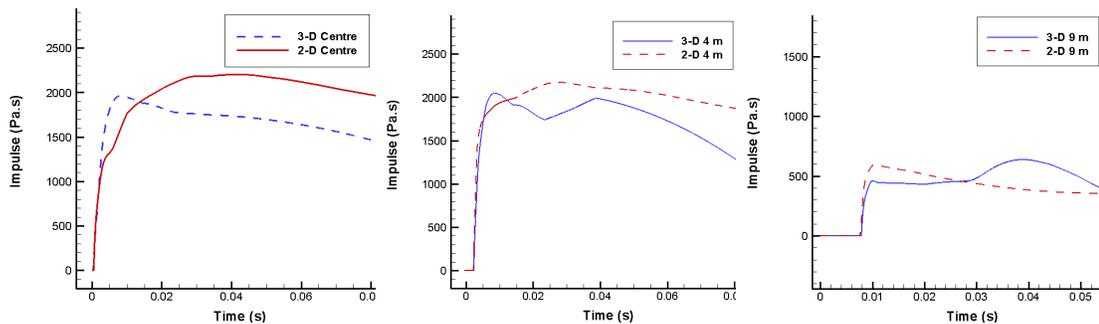
Figure 10. Comparison of pressure impulse (propane-air mixture) at 3 monitoring points between the pancake (solid-red line) and hemispherical clouds (blue-dashed line)
