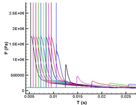
Figure 7. Pressure diagram for propane-air cloud, Pressure drop for pancake cloud [2]
