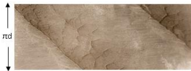
Fig. 5. Smoked foil records of a spinning detonation (6.35 mm annular channel, C_2H_2 + 5N_2O + 50\%Ar mixture).
