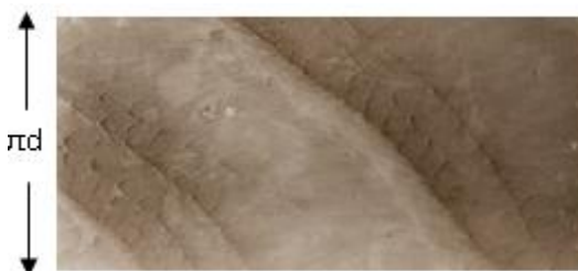
Fig. 6. Smoked foil records of a spinning detonation (3.175 mm annular channel, C_2H_2 + 2.5O_2 + 70\%Ar mixture).
