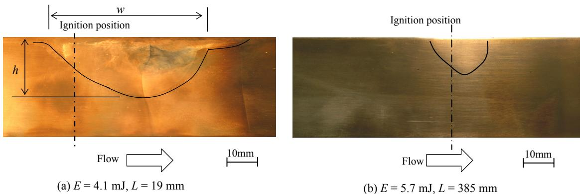
Figure 5. Soot record for spark discharge at initial pressure of 100 kPa
