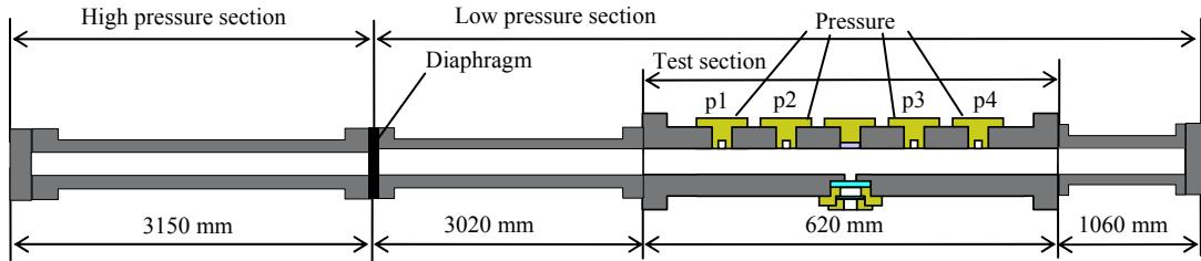
Figure 1. Schematic of shock tube
