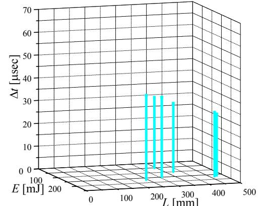
(b) A relationship of ignition energy, the distance from the incident shock wave to the ignition position, and the time from the ignition timing to the detonation origin. Laser ablation at initial pressure 35 kPa; shock Mach number  $Ms = 2.4 \pm 0.1$ ,  $T_2 = 525 \pm 25$  K,  $P_2 = 2.4 \pm 0.3$  atm.
