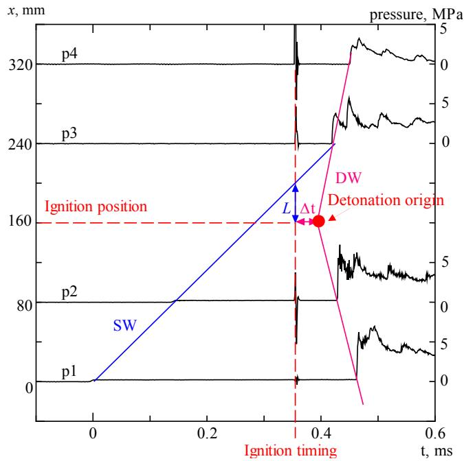
Figure 3. Pressure histories and  $x$ - $t$  diagram. SW: incident shock wave. DW: detonation front.  $\Delta t$ : time from ignition timing to onset of detonation.  $L$ : distance from the incident shock wave to the ignition position.
