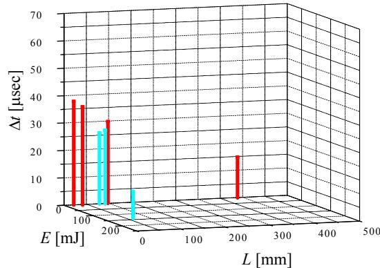
(c) Comparison of ignition methods (spark discharge and laser ablation). Initial pressure 100 kPa; shock Mach number  $Ms = 1.7 \pm 0.1$ ,  $T_2 = 400 \pm 20$  K,  $P_2 = 3.3 \pm 0.4$  atm.
