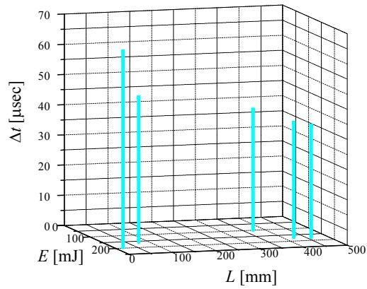
(a) A relationship of ignition energy, the distance from the incident shock wave to the ignition position, and the time from the ignition timing to the detonation origin. Laser ablation at initial pressure 25 kPa; shock Mach number  $Ms = 2.4 \pm 0.1$ ,  $T_2 = 530 \pm 20$  K,  $P_2 = 1.7 \pm 0.2$  atm.
