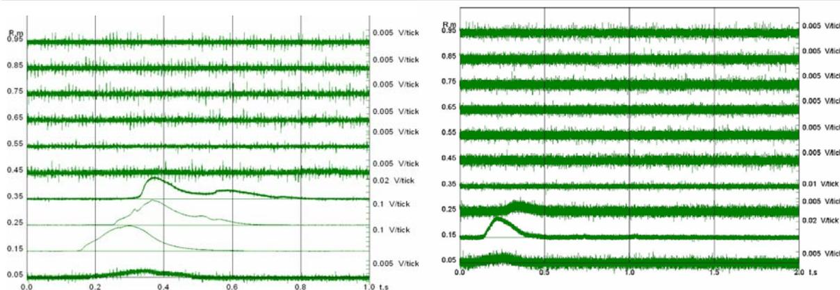
Figure 4. X-t diagram of combustion decay for 11% addition of  $C_2F_4Br_2$  and  $T=23^\circ C$  (left) and for 14% addition of  $C_2F_4Br_2$  and  $T=120^\circ C$  (right) in a small scale tests.
