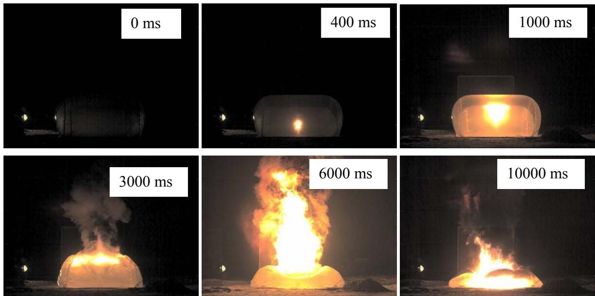
Figure 6. Combustion of stoichiometric hydrogen-air mixture with addition of 8.5%  $C_2F_4Br_2$  phlegmatizator. High-speed video record frames.
