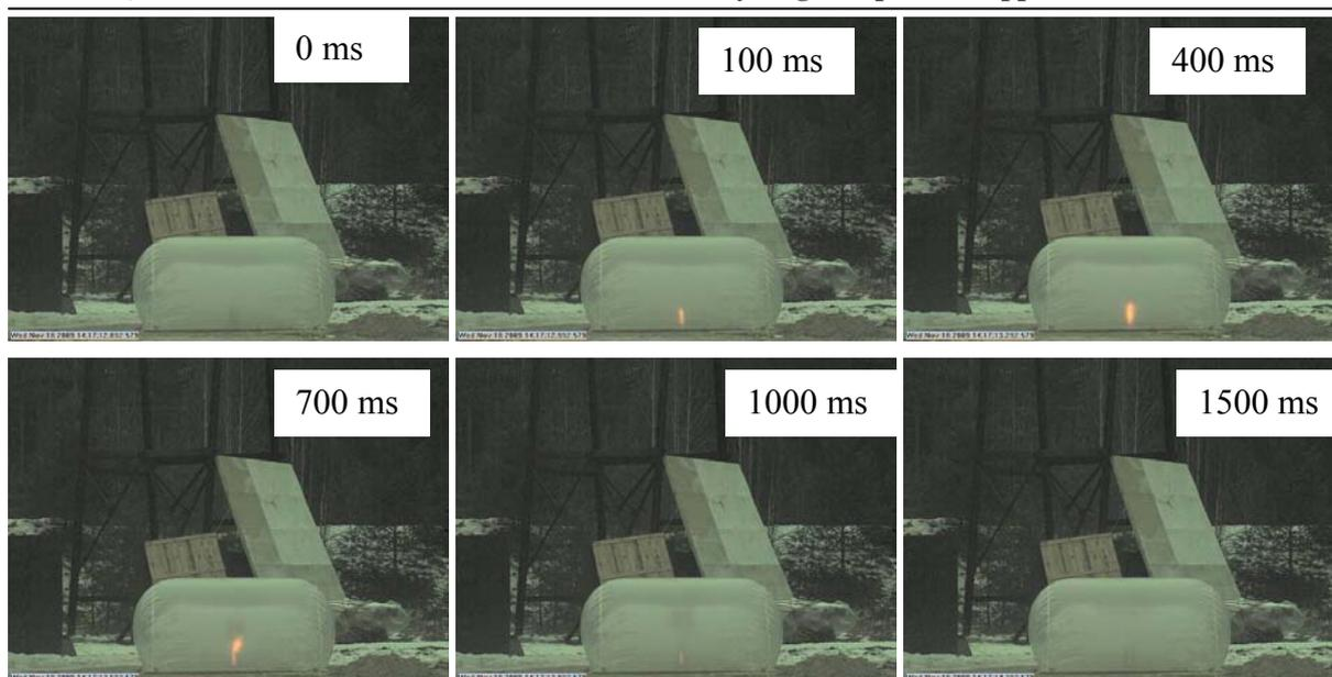
Figure 7. Full combustion suppression of stoichiometric hydrogen-air mixture with addition of 10.4%  $C_2F_4Br_2$  + 1.7%  $C_2F_3Cl_3$  phlegmatizer mixture. High-speed video record frames.
