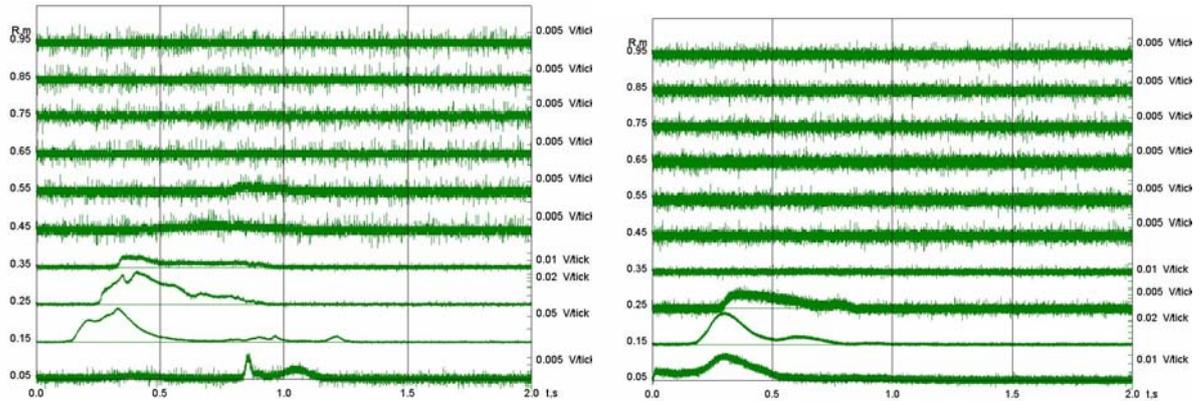
Figure 5. X-t diagram of combustion decay for 9%  $C_2F_4Br_2$  + 2%  $CF_3I$  and  $T=27^\circ C$  (left) and for 10%  $C_2F_4Br_2$  + 3%  $CF_3I$  and  $T=120^\circ C$  (right).
